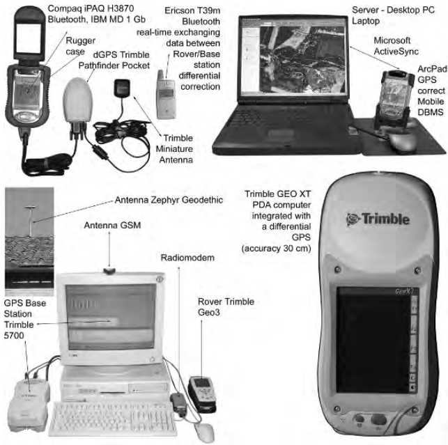
Figure 9. PDA, mobile GIS/GPS and DBMS solution tested during our landscape projects.
