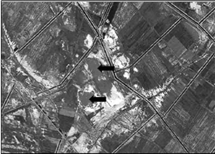
Figure 6. Examples of the types of features studied in the investigations. In the Landsat TM Band 3 image (1:7,000) above, various types of linear and curvilinear features denote relict drainage ways. The arrow at “1” indicates a relict river meander loop. The arrow at “2” shows an additional relict channel while the arrow at “3” points to a recent irrigation canal. (below) SPOT Panchromatic image (1:18,000) of the site of Abu Salabikh. The arrows point to two of the site’s mounds. (SPOT image courtesy of NGA).
