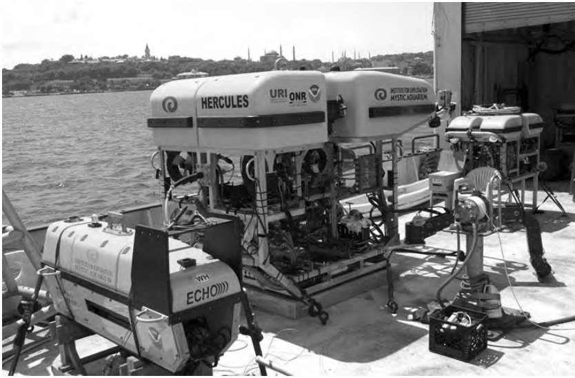
Figure 1. IAO's side-scan sonar vehicle ECHO (left), HERCULES ROV (middle), and LITTLE HERC ROV (right).
