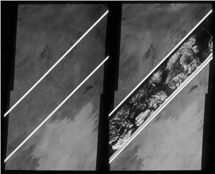
Figure 3. Landsat MSS image (left) with the coverage of the Space-borne Imaging Radar (SIR-A) image strip (right) superposed. The images cover part of the Darfur region of northwestern Sudan. The radar wave penetrated the sand cover to reveal the courses of three major dry rivers: the largest one in the upper right part of the strip is 20 km across. Source: Elachi and Granger, 1982.
