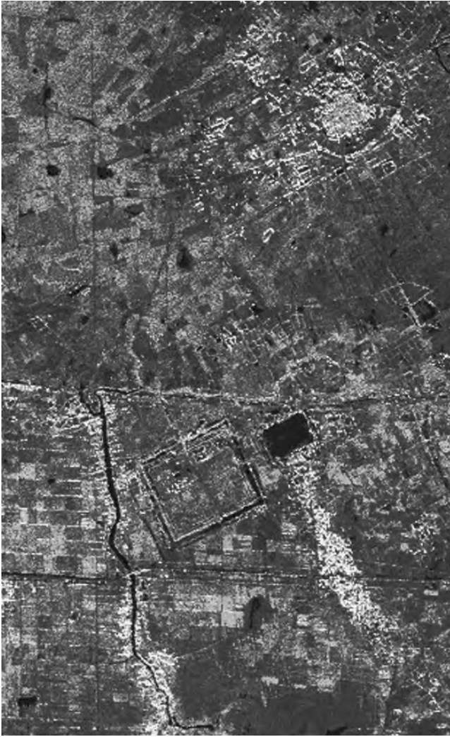
Figure 11. P-Band image of Lovea and Banteay Sras, west of Angkor (see also Figure 7). The circular earthwork and moat, as well as the elevated central mound of Lovea, appear as bright patterns on this image generated from P-Band data acquired during the 1996 AIRSAR acquisition. South (left) of Lovea is the rectangular enclosure of the later temple of Banteay Sras. Both are aligned to optimize water control on the slight northeast to southwest slope of the Angkor floodplain.
