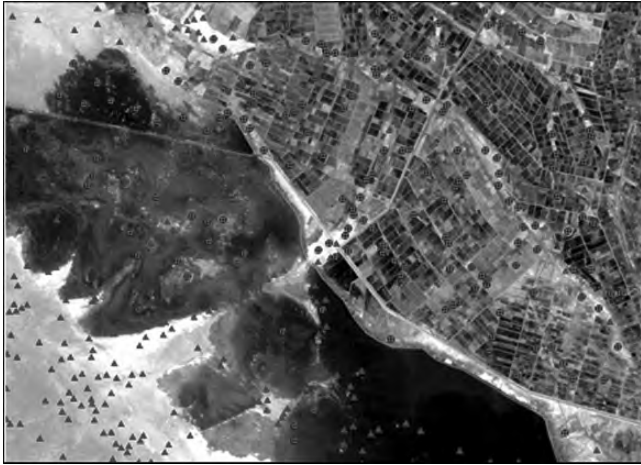
Figure 24. On this portion of a Landsat TM image (1:53,600) the blue triangle symbols represent the location of sites taken from the Adams' survey. The red circles represent additional potential sites that have been identified through digital image processing and interpretation. It should be noted that none of these new sites has been verified on the ground.
