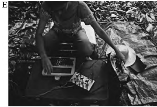
Figure 1 (Continued). Geophysical equipment used in the Lower Amazon Project. A. Proton magnetometer, Teso dos Bichos mound. B. Ground-penetrating radar, Teso dos Bichos mound. C. EM 31 Conductivity meter. D. Seismic refraction, Guajara mound. E. Electrical resistivity, Guajara mound. Photos by A. C. Roosevelt.
