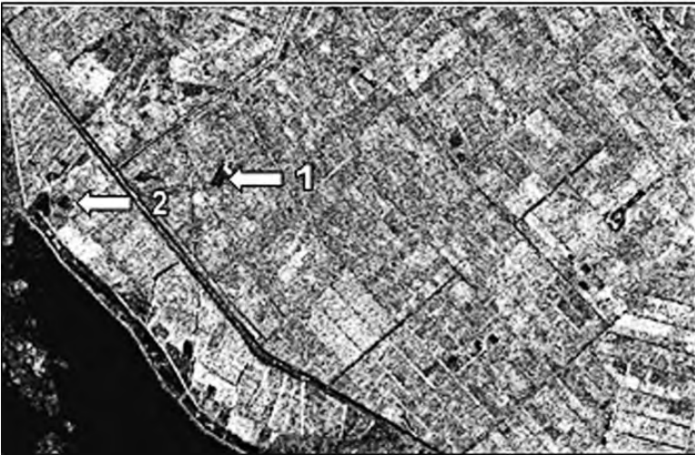
Figure 22. Area of irrigated agriculture east of Lake Dalma. (above) Landsat TM Band 3 image (1:20,000). A relict site is located at "1." Note the area at "2" with its bright reflectance, where other sites are located, b) Radarsat image (1:18,500) covering the same area. The black areas indicate small amounts of backscatter from level areas. These areas probably represent sites with little relief or prominent structures. Note how detail in the bright area at "2" in the image below can be discriminated better on the radar image. (RADARSAT image courtesy of EODS).
