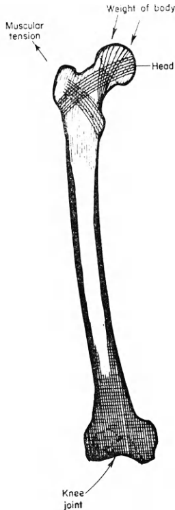
FIG. 7. Diagram of a section through the human femur, to show the orientation of trabeculae along the main lines of stress.
