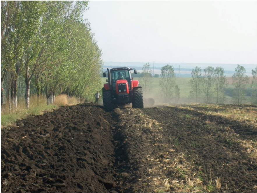
Fig. 4 Drawing the mouldboard plough at the experimental fields of Selectia Research Institute for Field Crops at Balti
