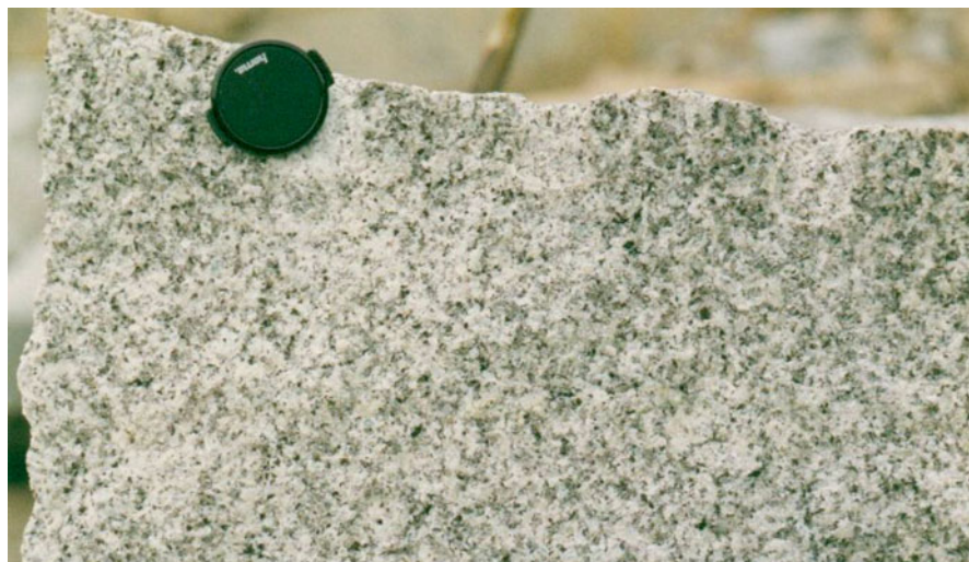
Fig. 2.3a Tin Granite (Granite No 4), the most strongly fractionated granite shown in its normal or un-mineralized facies. Kugler Quarry near Tröstau, Fichtelgebirge-Germany. Lens-protection for scale
