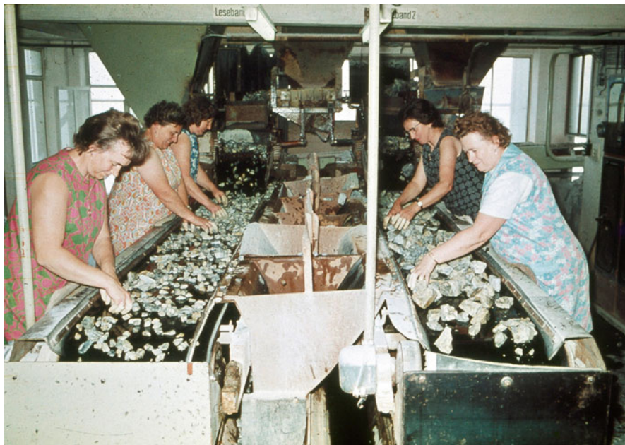
Fig. 1.4d Female workers sorting the high-quality feldspar by hand and picking the trash on the conveyor belt at Hagedorf-South (Courtesy of E. Keck 1990)
