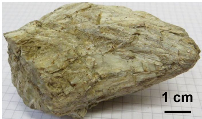
Fig. 5.2a Bundles of pale white wollastonite make up the hornfels at the Galgenberg area to the W of Pleystein
