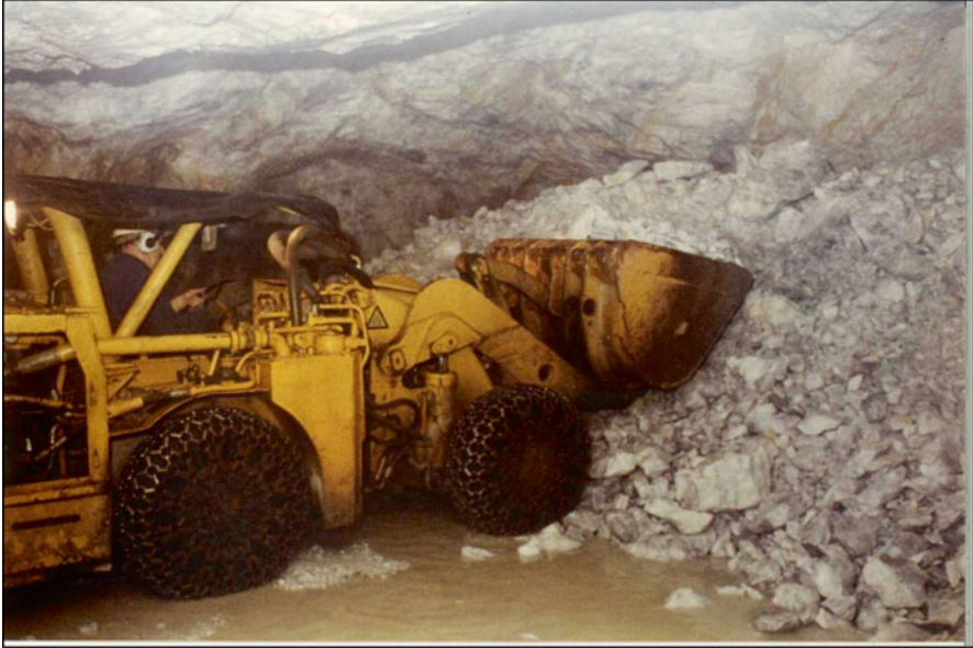
Fig. 1.41 A front-end-loader manned by one driver in the underground extraction site of the aplite mine—see the white rock on the roof and the blasted feldspar “ore” piled up in the foreground
