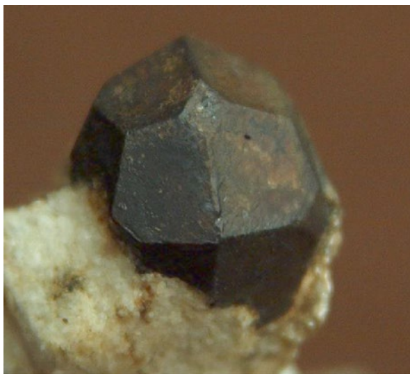
Fig. 4.3d Almandine garnet from the metapegmatite of the Wilma deposit near Püllersreuth (Weber 1978a) size: 2 cm
