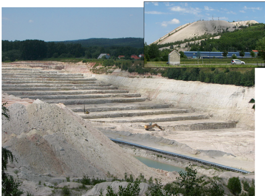
Fig. 1.5d Lower Triassic arkoses (Buntsandstein) enriched in kaolin and feldspar are currently more competitive than the pegmatitic ore bodies. Two industrial minerals can be extracted from the large open pits in the Hirschau-Schnaittenbach area, while quartz is dumped and form the “Monte Kaolino” which is the basis for a recreation center and leisure site to practice summer skiing and operate a toboggan run (See inset)
