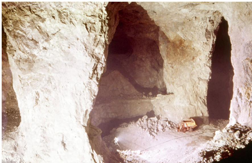
Fig. 1.4c Viewing the pillars and the chambers in the feldspar zone at the 87 m-level of Hagendorf-South Mine. For scale see the overhead- loader at the foot of a pillar and the flood light near the pillar on the left-hand side (Courtesy of E. Keck 1990)
