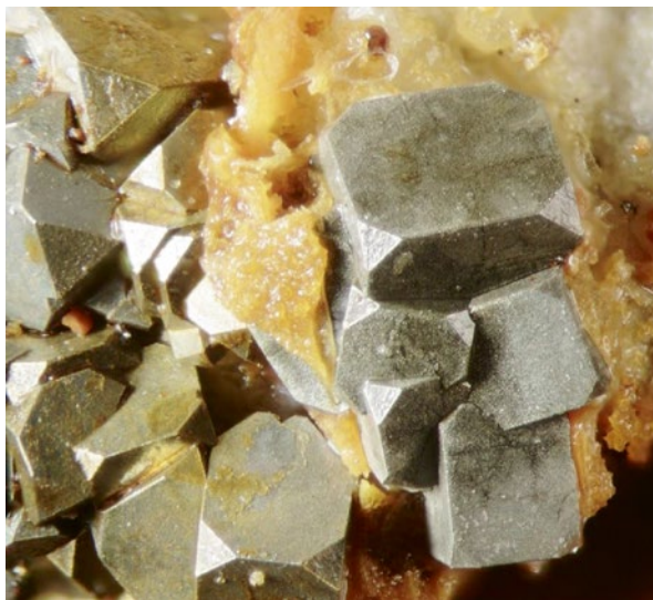
Fig. 4.15f Intergrowth of pyrite crystals giving rise to a face combination with hexahedron prevailing over the octahedron. Hagendorf-South
