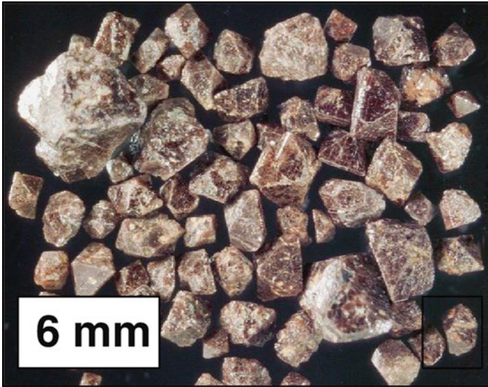
Fig. 4.5a Bipyramidal opaque brown zircon grains in stream sediments of fluvial placers concentrated by panning. Locality: Pleystein-Lerau drainage systems
