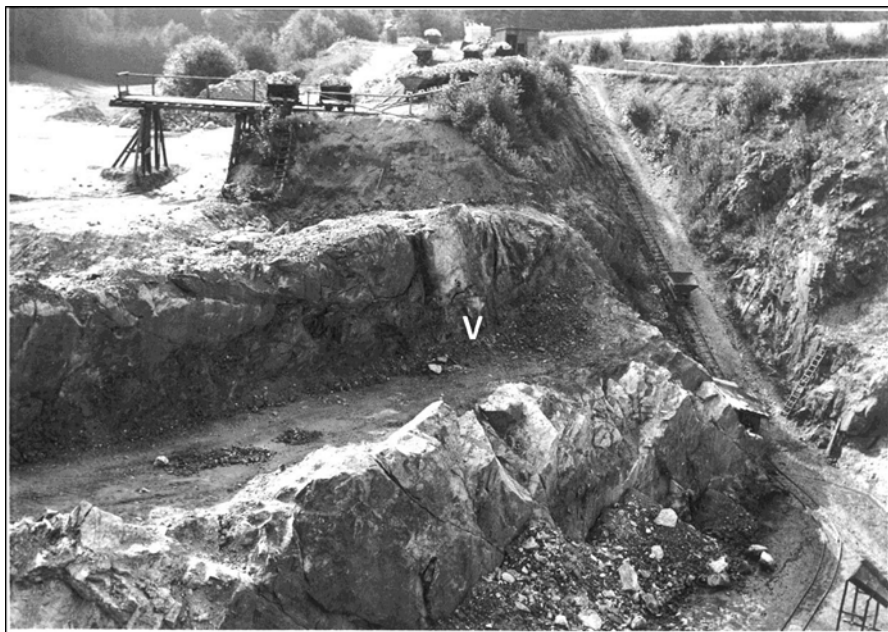
Fig. 1.6b Open pit mining of metapegmatites for feldspar near Wendersreuth during the initial phases of operation as the metapegmatite was opened up. The white feldspar body is exposed at the deepest level of the open pit. The upper working level exposed an off-shoot (v) of the metapegmatite into the gneissic country rocks. The feldspar is transported out of the open pit by means of track-mounted mine cars of two-ways dumping type to the loading bridge, where the feldspar is handed over on to lorries (Courtesy of Gottfried Feldspat GmbH)
