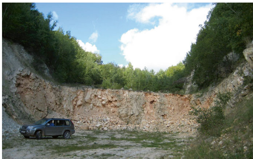
Fig. 2.1e Cross section through a massive quartz vein surrounded by Devonian slates and operated in an open pit near Usingen, Germany, for high-purity quartz
