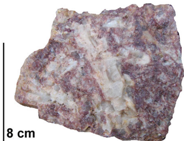
Fig. 2.4a Slender crystals of albitic feldspar in a matrix of lepidolite. Rožna pegmatite, Czech Republic
