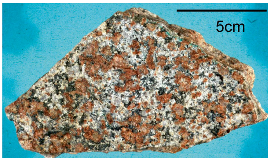
Fig. 2.3b Tin Granite (Granite No 4). Specimen has been taken from the mineralized facies or greisen facies with cassiterite ( black ) and corroded arsenopyrite. Rudolfstein, Fichtelgebirge-Germany
