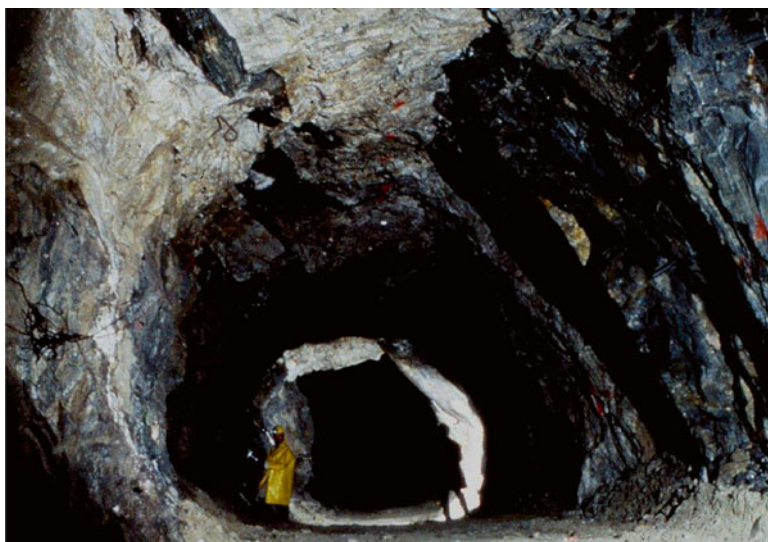
Fig. 1.2a Overview of the lithium pegmatites of the Koralpe Li deposit (Courtesy of R. Göd 1989). Adit exposing a lit-par-lit structure of aplitic and pegmatitic layers ( white ) and amphibolite ( dark )
