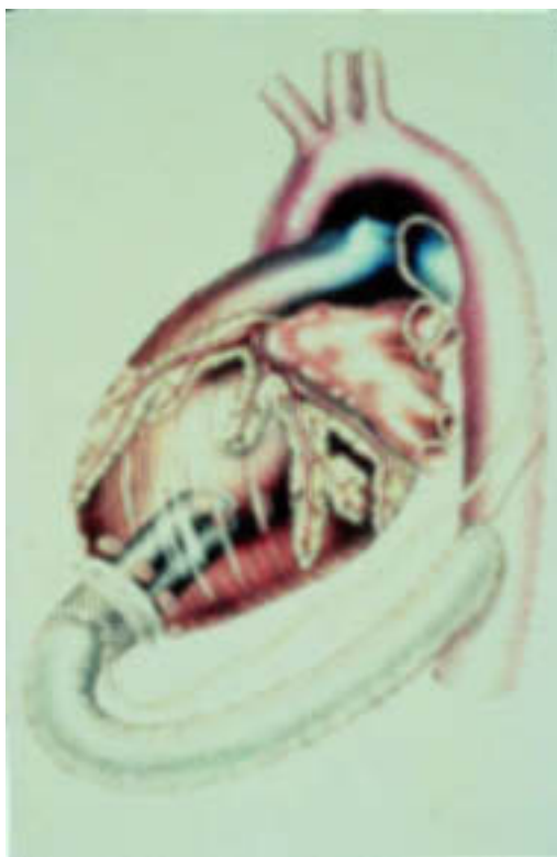
Figure 11.8. The intraventricular “Jarvik 2000 Heart”, an axial flow impeller pump which rotates at between 8000 and 18 000 rpm without damaging the blood.
