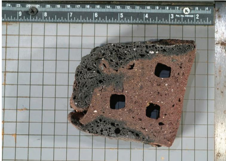
**Figure 4.1.1.** Modern brick from Trujillo, Peru brickyard showing bubbling, vitrification, and flow features caused by the 1300–1600°C coal-fired, curing process. Photo by William E. Brooks, 2006.
