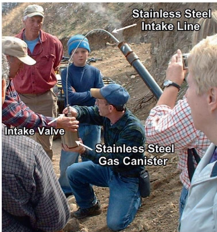
**Figure 9.2.8.** Gas collection technique using a stainless steel canister, South Canyon, Colorado. G.B. Stracher extracting coal-fire gas from a borehole into a fire in an underground coal-mine tunnel at the South Cañon Number 1 Coal Mine fire, Colorado. Photo by Janet L. Stracher, 2004.
