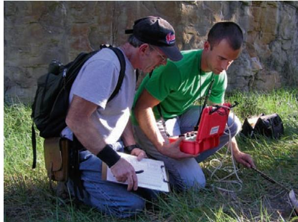
**Figure 9.2.11.** Pitot instrumentation (tube and flow meter (red box)) used for measuring the velocity of coal-fire gas exhaled from vents at the surface. This instrument is a product of FlowKinetics LLC, 528 Helena Street, Bryan, Texas 77801, USA. Photo by Jennifer M.K. O’Keefe, 2009.
