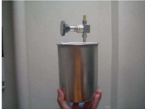
**Figure 8.1.1.** Sampling canister.
