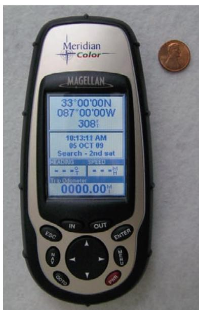
**Figure 9.2.4.** Magellan<sup>®</sup> handheld GPS unit. This model is waterproof and includes a backlit screen for readability on a cloudy day or after sunset. Similar units are offered by other manufacturers. Photo by Glenn B. Stracher, 2009.
