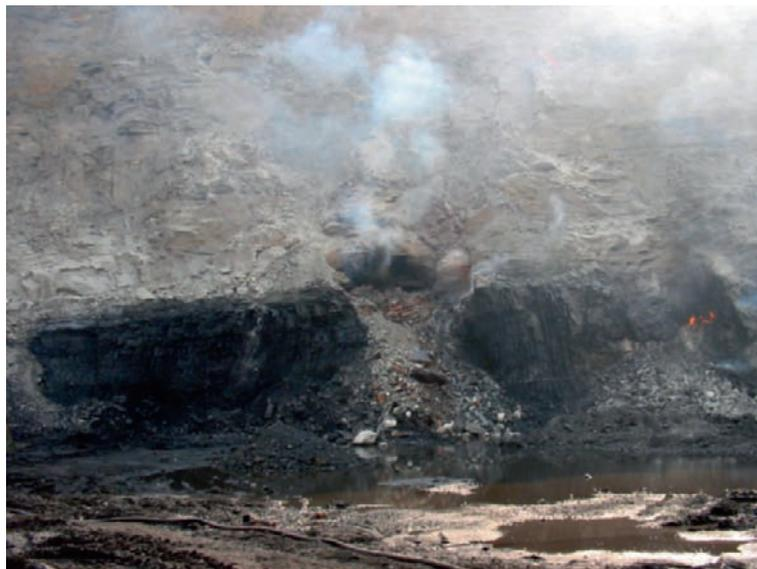
**Figure 6.1.4.** Coal fire in an open-pit mine in the Jharia coalfield, India. People who work in such mines are exposed to toxic gases, particulate matter, and the risk of ground subsidence. Photo by Prasun Gangopadhyay, 2006.
