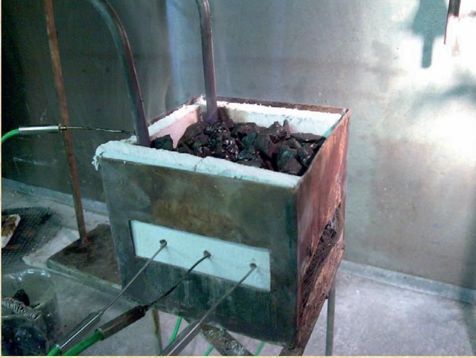
Small scale apparatus developed to study the burning characteristics and suppression of smoldering coal. *Photo by Rory Hadden, 2009.*
