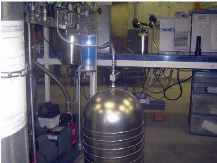
**Figure 8.1.7.** Whole air standard used for calibration on the VOC system.
