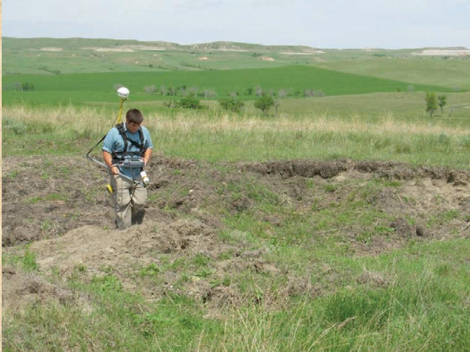
Andrew Sparks measuring the strength of the geomagnetic field with a cesium vapor magnetometer at the location of the Roedeske 4 burning coal seam in western North Dakota, USA. *Photo by Rob Sternberg.*
