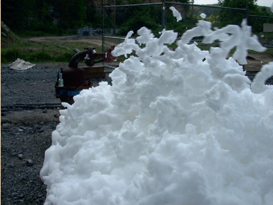
Compressed-nitrogen foam used to extinguish an underground coal fire at the Buchanan No. 1 Mine, Clay Pool Hill, Virginia. A pressure-relief bore hole in the photo is releasing compressed-nitrogen foam from a foam-filled mine cavity (gob and entries). This bore hole was located ~914 m horizontally from the original injection bore hole, at a depth of ~884 m. *Photo by Mark Cummins, 2007.*
