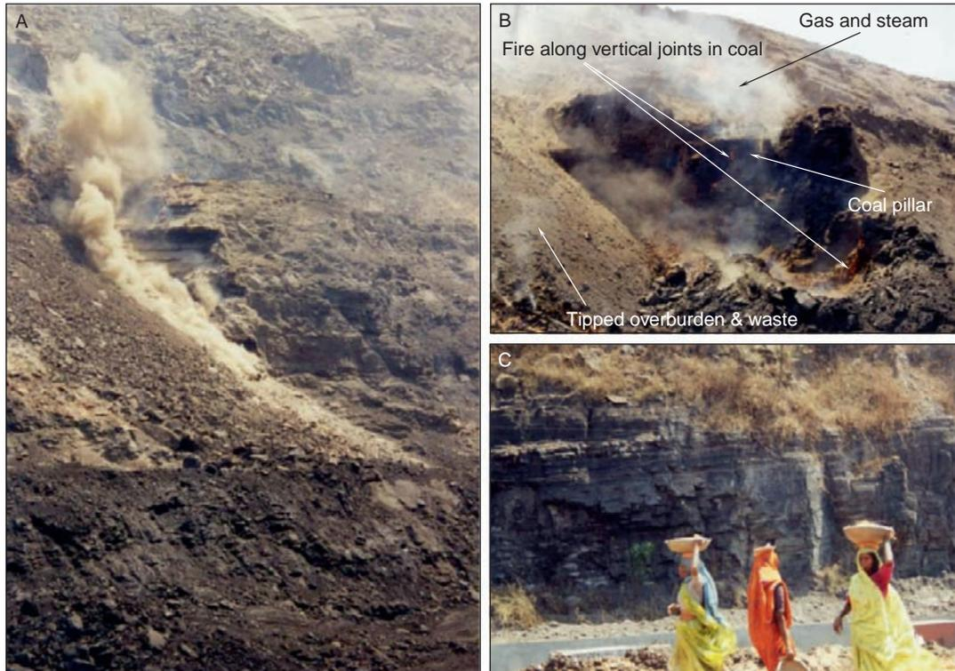
**Figure 5.1.7.** (A) Pillar failure caused by the spontaneous combustion of support pillars in an opencast coal mine. (B) Burning-coal pillars causing the failure of tipped material. (C) Smoldering and burning coal carried by local villagers, Singrauli coalfield, India. Photo A reproduced with permission of Taylor & Francis. Photo by Donnelly 2000.
