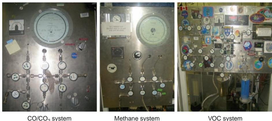
**Figure 8.1.3.** Gas-handling manifolds for the three analytical systems.
