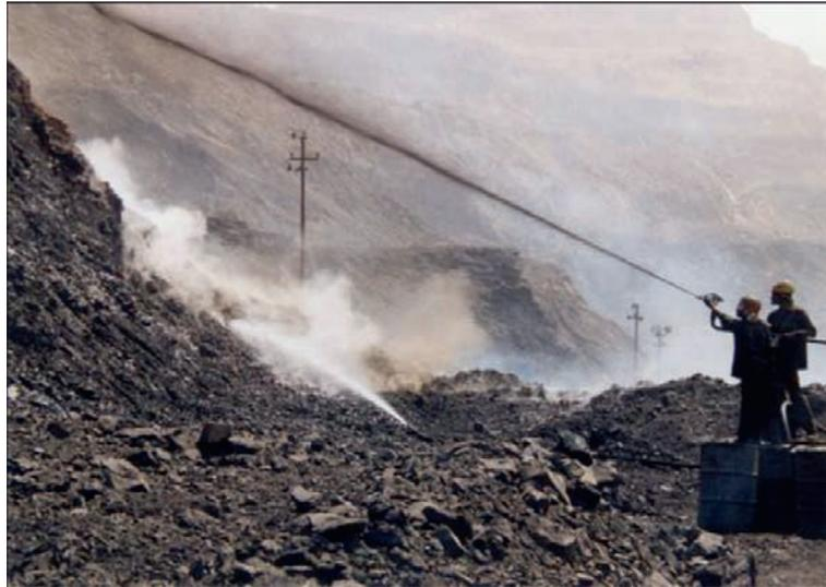
**Figure 5.1.4.** Fires extinguished by first spraying with water and then with a bitumen compound at high pressure to seal fissures and prevent air ingress (operated by two specially trained fire fighters). Reproduced with permission of Taylor & Francis. From Bell and Donnelly 2006; photo by Donnelly 2000.
