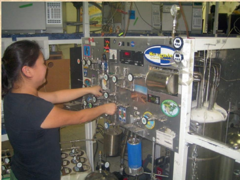
Gloria Liu in the process of preconcentrating a coal-mine-gas sample preparing for injection it onto the separation columns. *Photo by Timothy R. Blake, 2007.*
