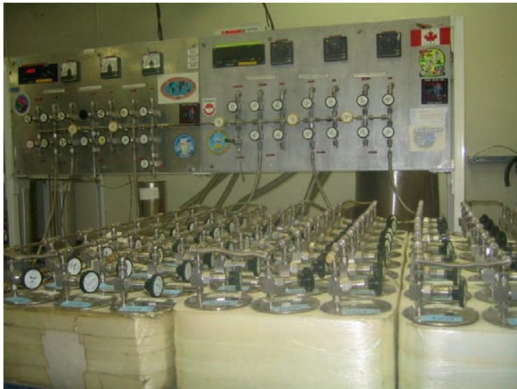
**Figure 8.1.2.** Canister evacuation pump-out vacuum line.
