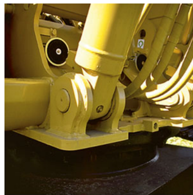
This pin is used to support the end of the strut used on a tractor. (8)
