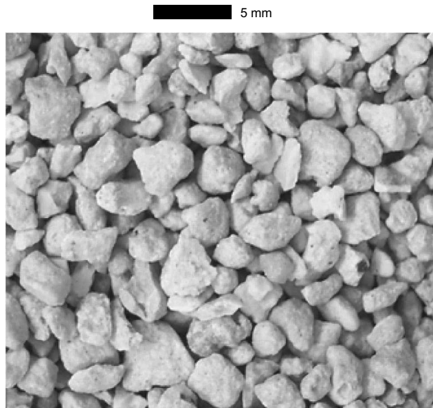
Fig. 1. Photograph of the granular expansive material with a maximum pellet size of 4 mm
