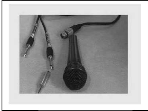
Figure 9.4 Cables from left: large jack, large jack with large to mini jack converter XLR
