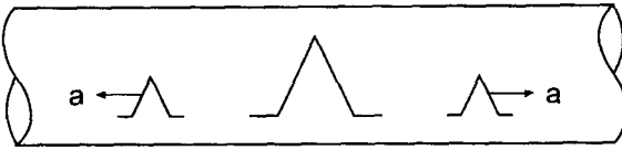
Figure 11.27 Acoustic wave propagation in an infinite duct.
