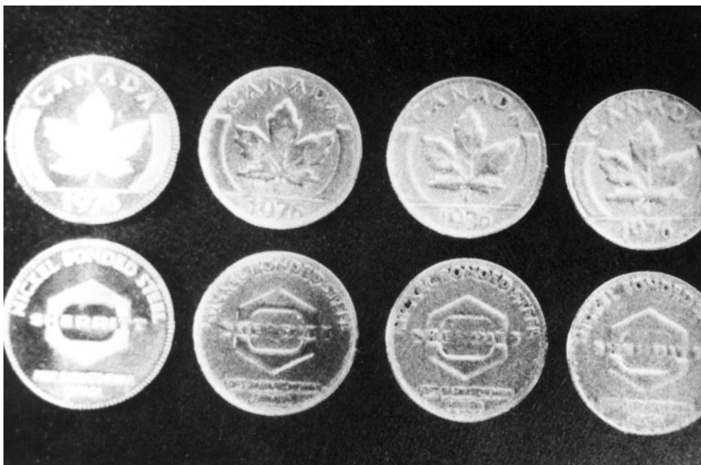
Figure 9.76 Examples of coins worn in the tumbling apparatus. (From Ref. 126, reprinted with permission from ASME.)
