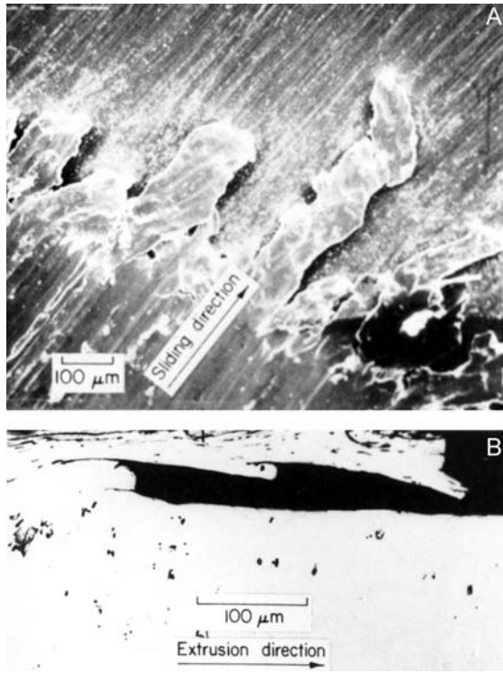
Figure 3.31 Crack structure in extrusion wear. In “A”, the surface morphology of the wear scar is shown. In “B”, a view of the cross-section through the wear scar. (From Ref. 87, reprinted with permission from ASME.)
