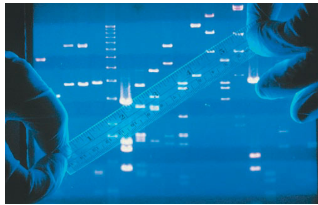
FIGURE 13–21 An agarose gel containing separated DNA fragments stained with a dye (ethidium bromide) and visualized under ultraviolet light. Smaller fragments migrate faster and farther than do larger fragments, resulting in the distribution shown.
