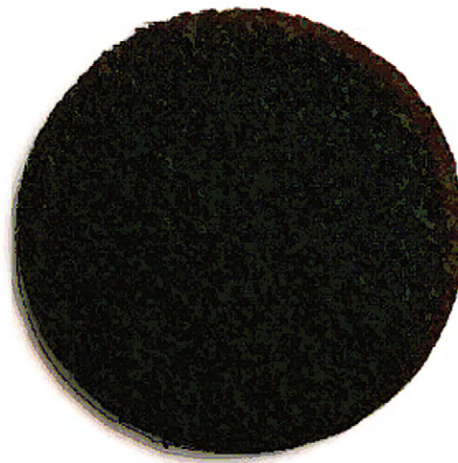
FIGURE 4B-2 Carbon pad, approximately 4 mm thick in discs up to 22 mm in diameter. Porosity is about 85%.
