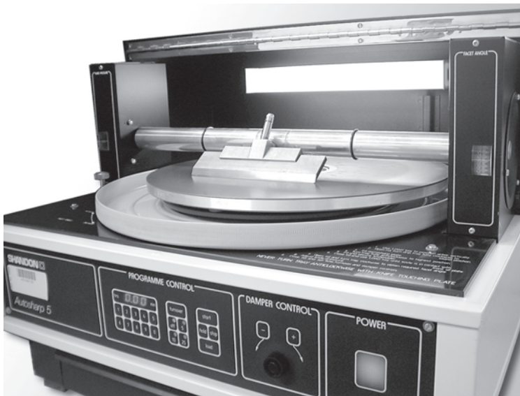
Fig. 2. Grinder used to sharpen the tungsten carbide blades.
