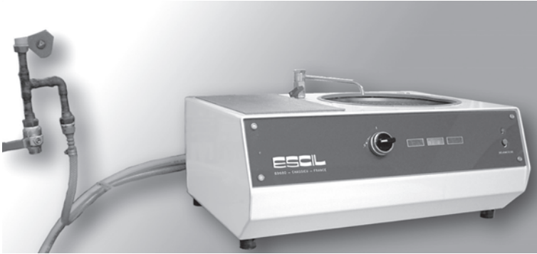
Fig. 1. Rotating wet-sander with an abrasive disc (working under running tap water), used to expose the embedded tibia along the right plane for cutting.
