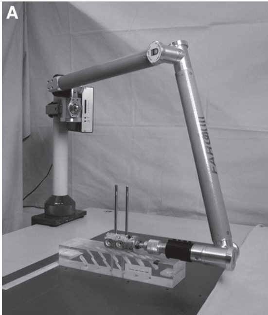
Fig. 1. FARO arm electrogoniometer (A) with probes for surface acquisition (B) and motion tracking (C) to be mounted at the last joint.
