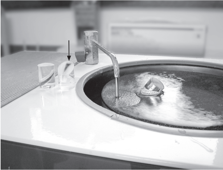
Fig. 4. Wet-sanding of an embedded tibia on the rotating sander. See a block eroded (arrow) along the right plane for cutting.
