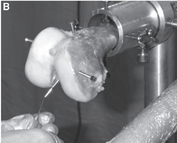
Fig. 3. Surface acquisition of tibia (A) and femur (B) during a knee study. Note that different probes can be used for the acquisition, and bones can be fixed in any convenient position.
