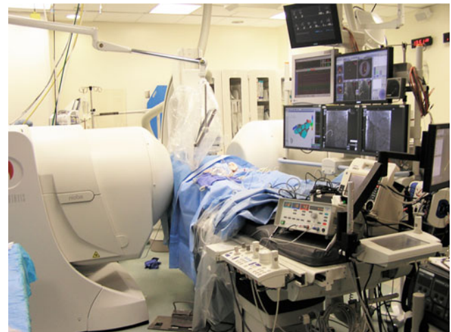
Fig. 21.2 The Niobe II system was approved for commercial release. It uses fixed magnets that are housed within the encasements positioned on either side of the patient
