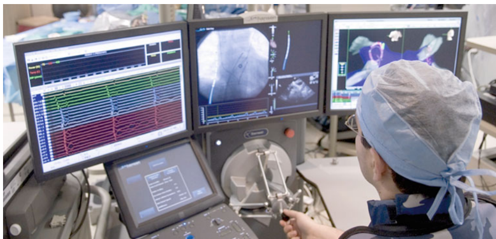
Fig. 21.9 The operator controls the robotic arm from a console at the workstation
