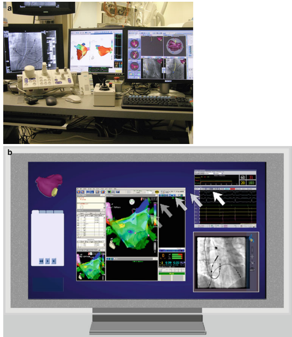
Fig. 21.3 (a) Computer interface with X-ray images, the CARTO electroanatomic image, and the Stereotaxis images are shown. The control box for the catheter advancer system is designated by an arrow . (b) An updated display, which is controlled by a single keyboard and mouse, integrates X-ray images, the CARTO image, and the Stereotaxis image on a single large plasma screen
