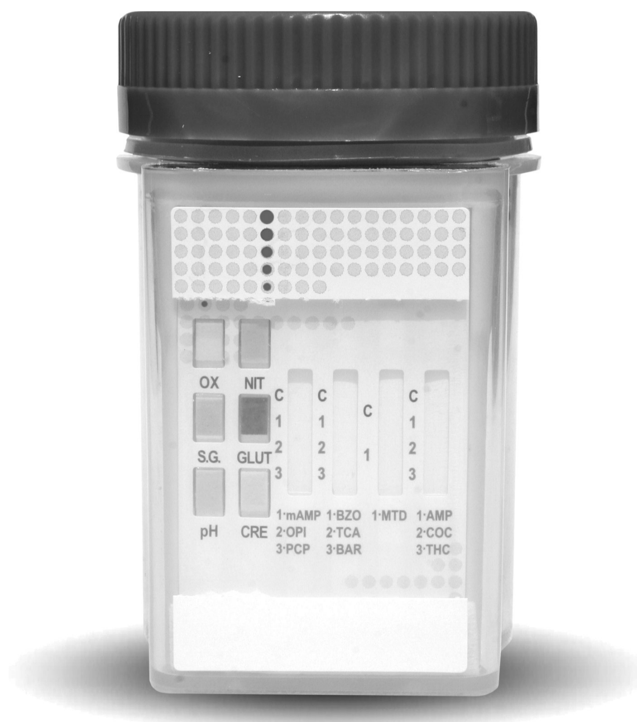
Figure 11.4. The i-Cup is an “all in one” urine sample collector and drug testing device. It detects the presence of drugs and adulterants (if present) in 5 minutes. Also, it measures the urine temperature (90°F–100°F) to prevent dilution during collection. The choice is from 14 drugs or drug classes that can be custom ordered in 3 to 10 drug panels. Positive samples can be sent directly to the laboratory for confirmation. The i-Cup also screens for adulterants: pH, specific gravity, and various oxidants. (Reproduced with permission from Instant Technologies, Norfolk, VA.)
