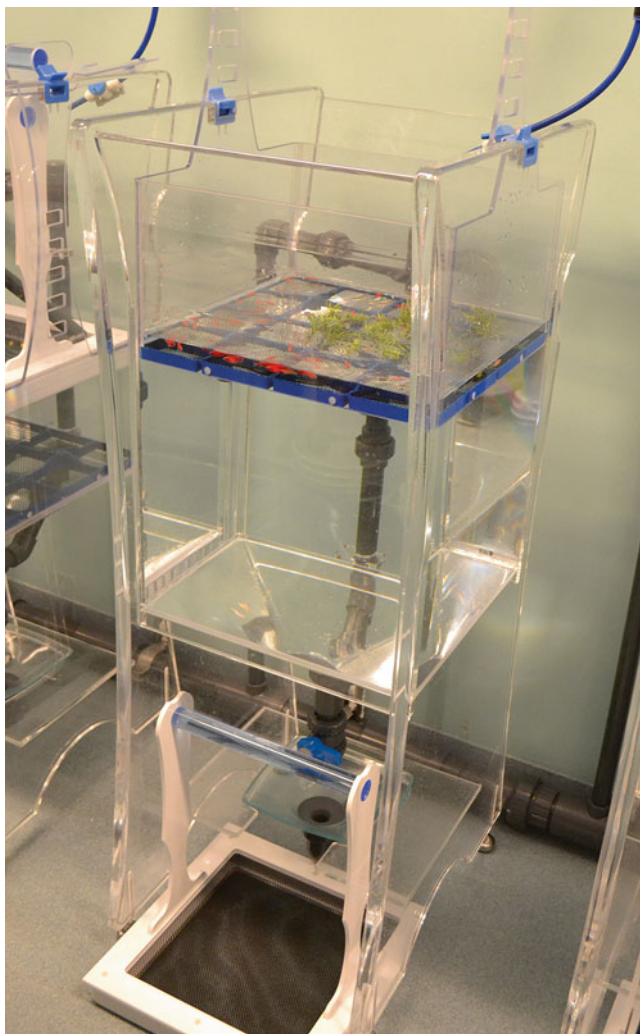
Fig. 2 The iSpawn is a specialized breeding tank designed to collect thousands of developmentally synchronous embryos. Approximately 200 adult zebrafish can breed in the shallow environment created by the mesh divider. Upwards of 10,000 embryos can be collected at the base of the vessel in minutes
