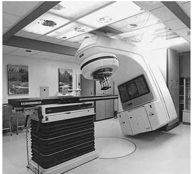
Figure 26-3 Linear accelerator. This Varian 2300 C linear accelerator can produce 6- and 18-MV photons as well as several energies of electron beam.
