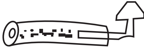
Fig. 8.16 The Zwaardemaker olfactometer and the Elsberg's blast injection apparatus for quantifying the exposure to an odorous stimulus
