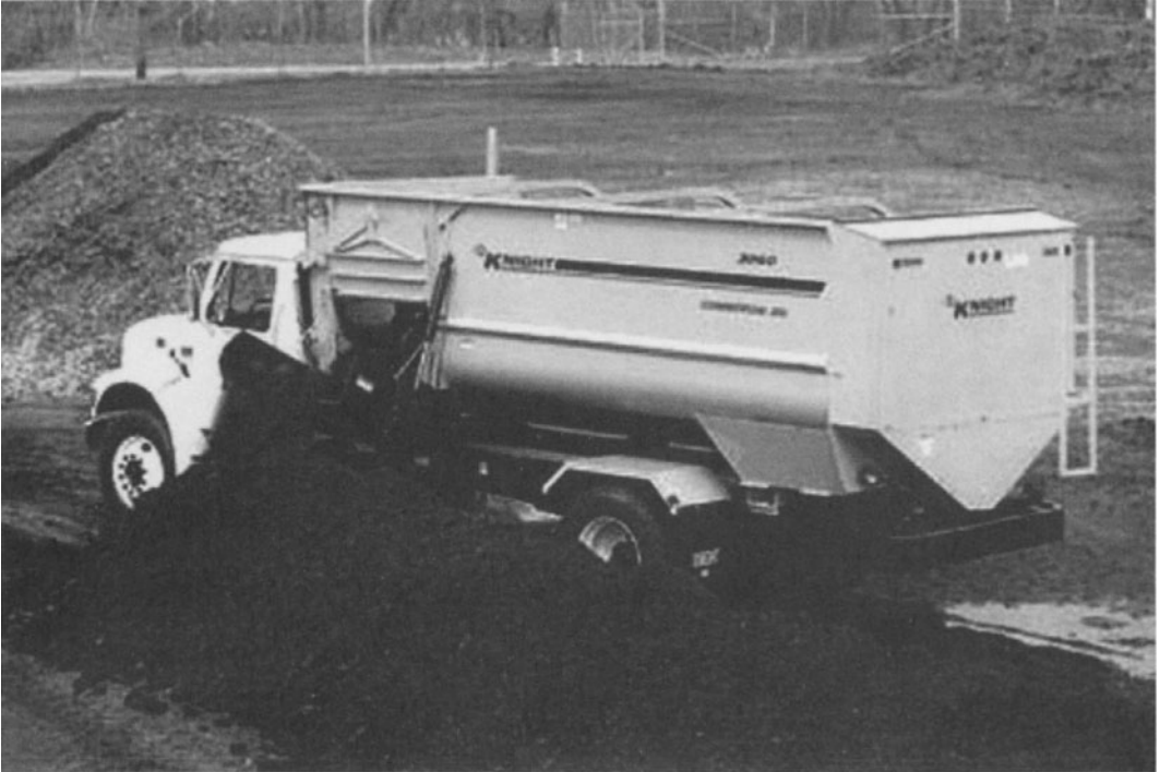
FIGURE 5.8 Photograph of a Knight Reel Auggie for soil mixing and distribution. Courtesy of Kuhn Knight.
