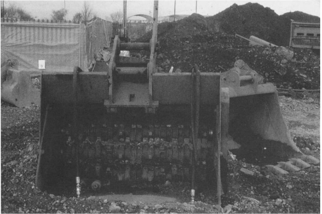
FIGURE 5.9 Photograph of an ALLU bucket. It is fitted with rotating drums with blades, and also crushing bars, so that it can be used to grade soil containing materials such as brick. Courtesy of WSP Remediation Ltd.
