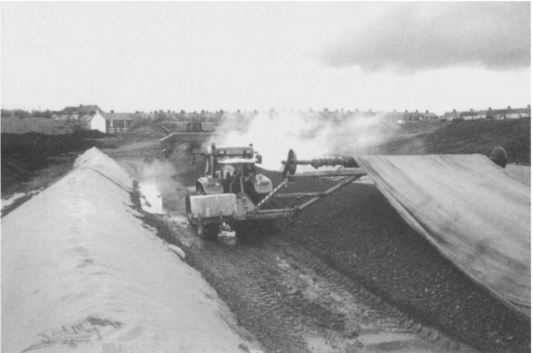
FIGURE 5.6 Photograph of a fleece roller. A self-propelled windrow turner can be seen in the background. Courtesy of Shanks Waste Management Ltd., United Kingdom.
