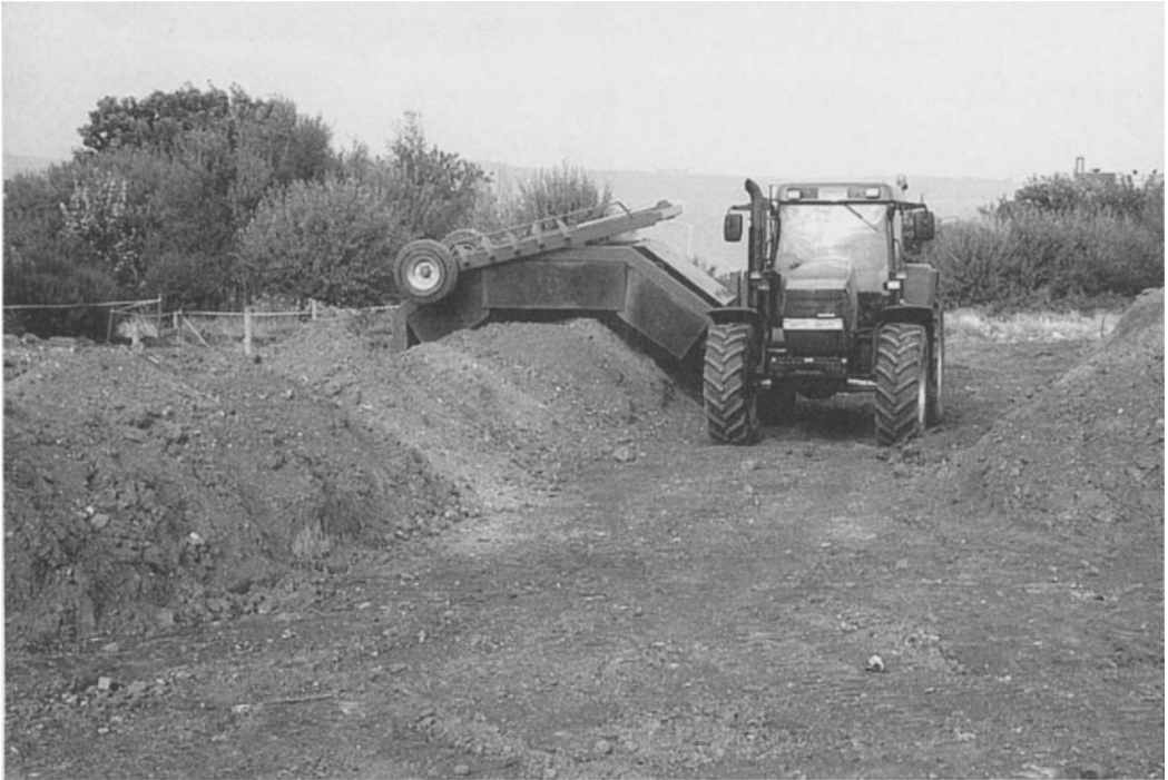
FIGURE 5.12 Photograph of a tractor-driven windrow turner. Courtesy of Environmental Reclamation Services Ltd., Glasgow, Scotland, United Kingdom.
