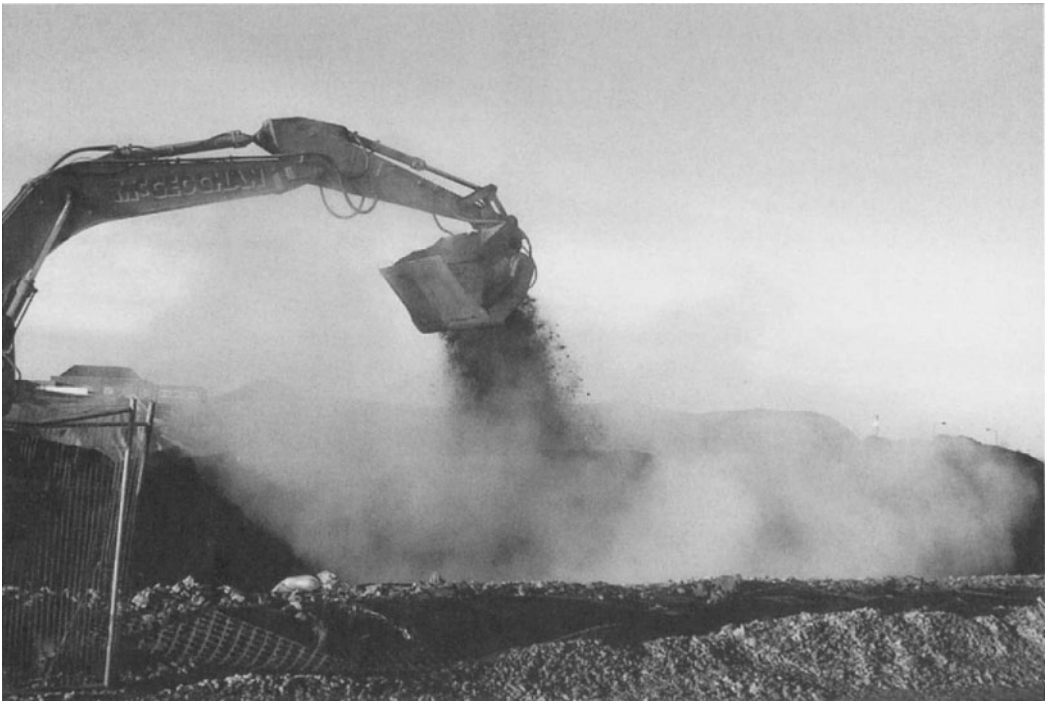
FIGURE 5.11 Photograph of an ALLU bucket being used as a windrow turner. Courtesy of WSP Remediation Ltd. Its adaptability to different machinery and its low cost make it a flexible alternative to windrow turners, although slower.
