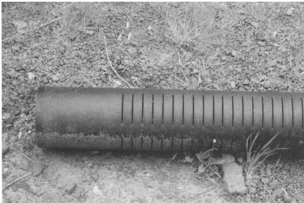
FIGURE 5.4 Photograph of a biopile slotted pipe (plastic pipe, 4-in. diameter).
