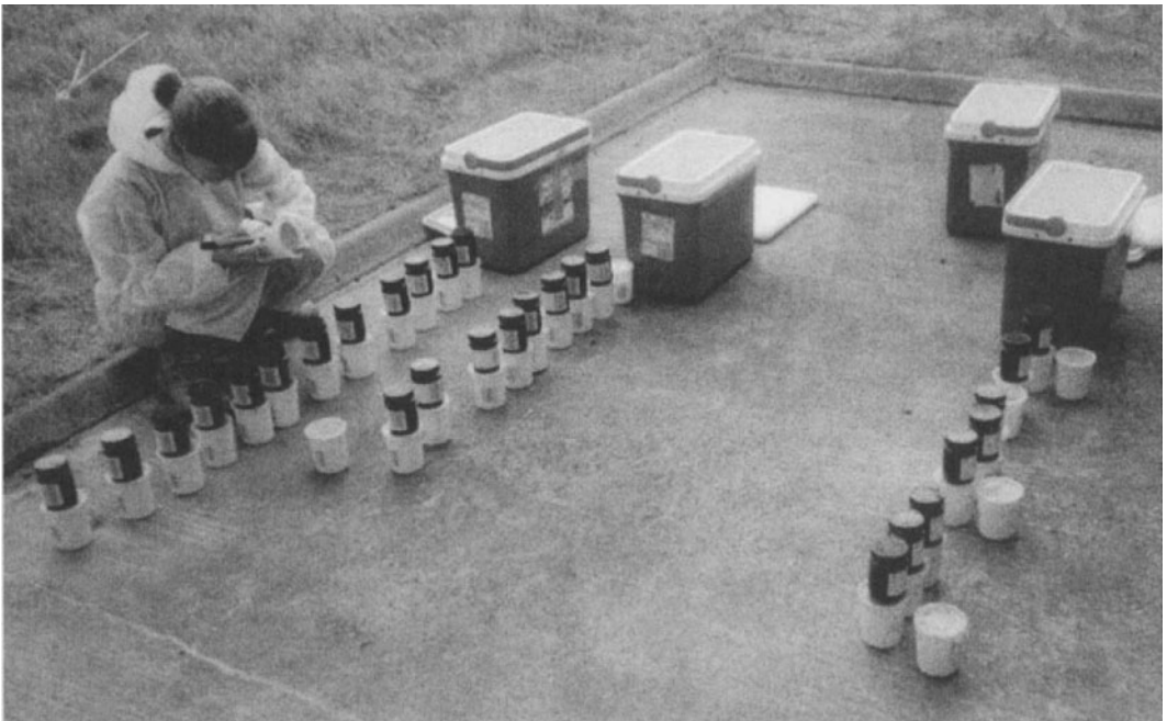
FIGURE 2.3 Scheduling of soil samples prior to laboratory analysis. The labeling procedure, often overlooked, should be viewed as an essential part of the overall procedure and should be given requisite attention to detail.
