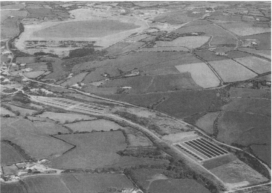
BOX FIGURE 8.4.1 Aerial photograph (above) of the Wheal Jane Mine in Cornwall, United Kingdom, and a schematic of the passive treatment processes (next page) installed for the bioremediation of mine wastewaters (with permission from CL:AIRE).
