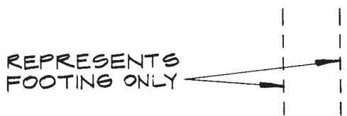
Figure 9.4B Plan view of interior nonbearing footing.
