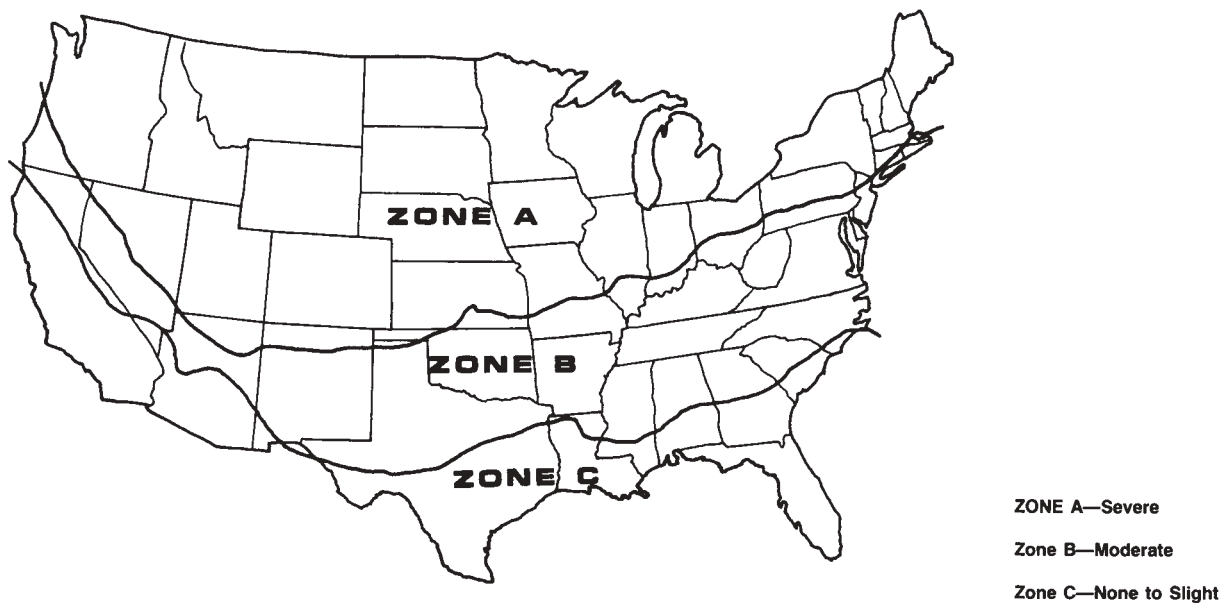
Figure 13.50 U.S. condensation hazard zones.
