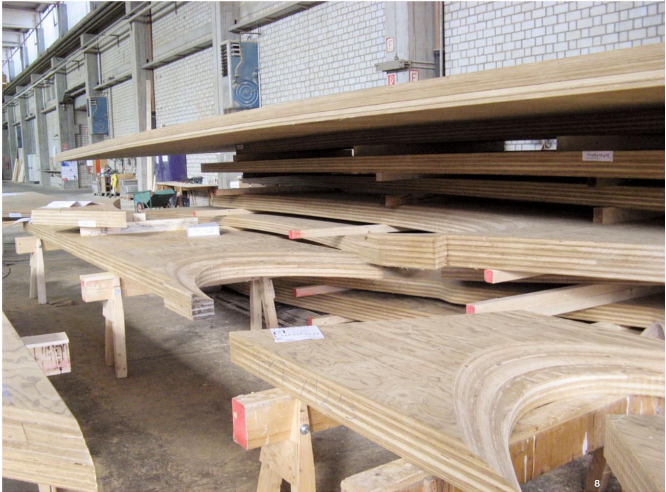
ments of the structure, the “Kerto-Q” wooden panels, with a maximum width of 69 mm, are glued together to make up composite panels of up to 224 mm and then preventively impregnated in a special high-pressure chamber.
