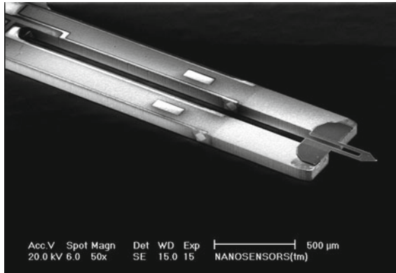
Fig. 18.3 SEM image of Akiyama probe. Copyright by NanoWorld AG
