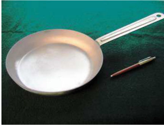
Fig. 13.1 A stainless steel pan coated by a quasicrystal material. The coating was made using electron beam vapor deposition in vacuum
