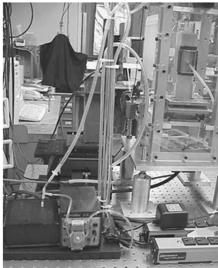
Figure 11.6 Photograph of the system shown in Figure 11.5. From the left are the pressure sensor and computer interface chassis, the peristaltic pump, and the manometer fluid column U tube.
