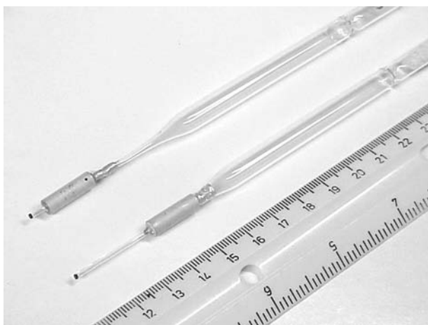
Figure 10.19 Photographs of cylindrical piezoelectric drive element drop ejectors detailed in Figure 10.18. Conductive epoxy is used to access the inner electrode and bond the drive element to the glass reservoir tube.
