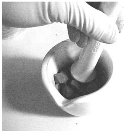
Figure 14.1 Crushing a fragmentable solid using a mortar and pestle. The initial fragmenting of materials solids for the purpose of producing an ejectable colloidal suspension can be implemented by a process as simple as mechanical crushing with a mortar and pestle. The typical mean particle diameters achievable by mechanical crushing is in the 10–100 micron range.
