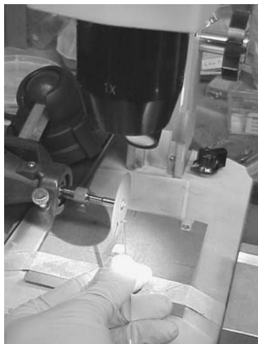
Figure 10.6 Trimming excess material from the welded orifice plate. Cutting away excess aperture plate material eases cleaning and improves mechanical ruggedness. A set up to perform this operation can be constructed from a motorized hand grinder such as a Dremel MotoTool spinning a disc of 400 grit carborundum paper. Precise grinding is facilitated by performing this operation under a binocular inspection microscope.
