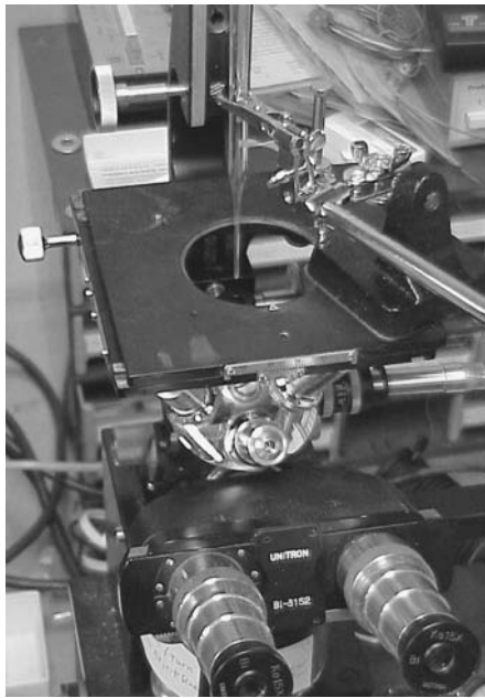
Figure 9.10 A microscope with a calibrated reticle is used to measure the diameter of the hole to determine when grinding back the tip should stop. The photo shows a Pasteur pipette with an thermally pulled ground back tip being inspected.
