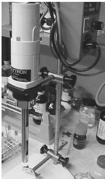
Figure 14.3 Rotary homogenizer (left) and details of the high shear rate mixing tip (right). High speed rotation of the rotor inside the slotted stator draws the fluid powder mixture into the inside of the stator where it is exposed to a high shear region between the rotor and the stator and is forced out the slots. The fluid shear between the rotor and stator accomplishes the necessary particle deagglomeration, wetting and dispersing.
