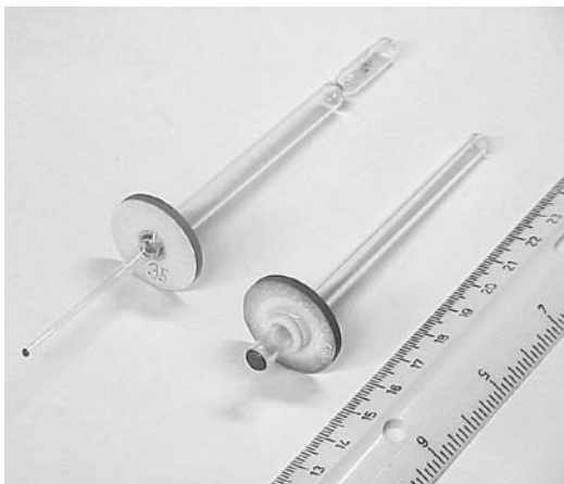
Figure 10.15 Photograph of glass body drop ejectors diagrammed in Figure 10.14.
