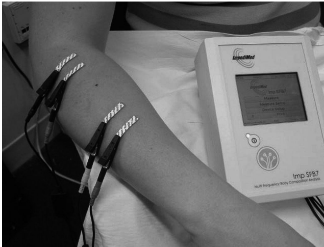
Figure 7-4. “Near-electrode” montage to study the extensor digitorum communis muscle. In this montage, the far right and far left electrodes are the current-injecting electrodes. The center electrodes are the voltage-sensing electrodes. (Adapted from Rutkove SB. Electrical impedance myography: background, current state, and future directions. Muscle Nerve . 2009;40(6):937. Copyright 2009 Wiley Periodicals. Reprinted with permission.)
