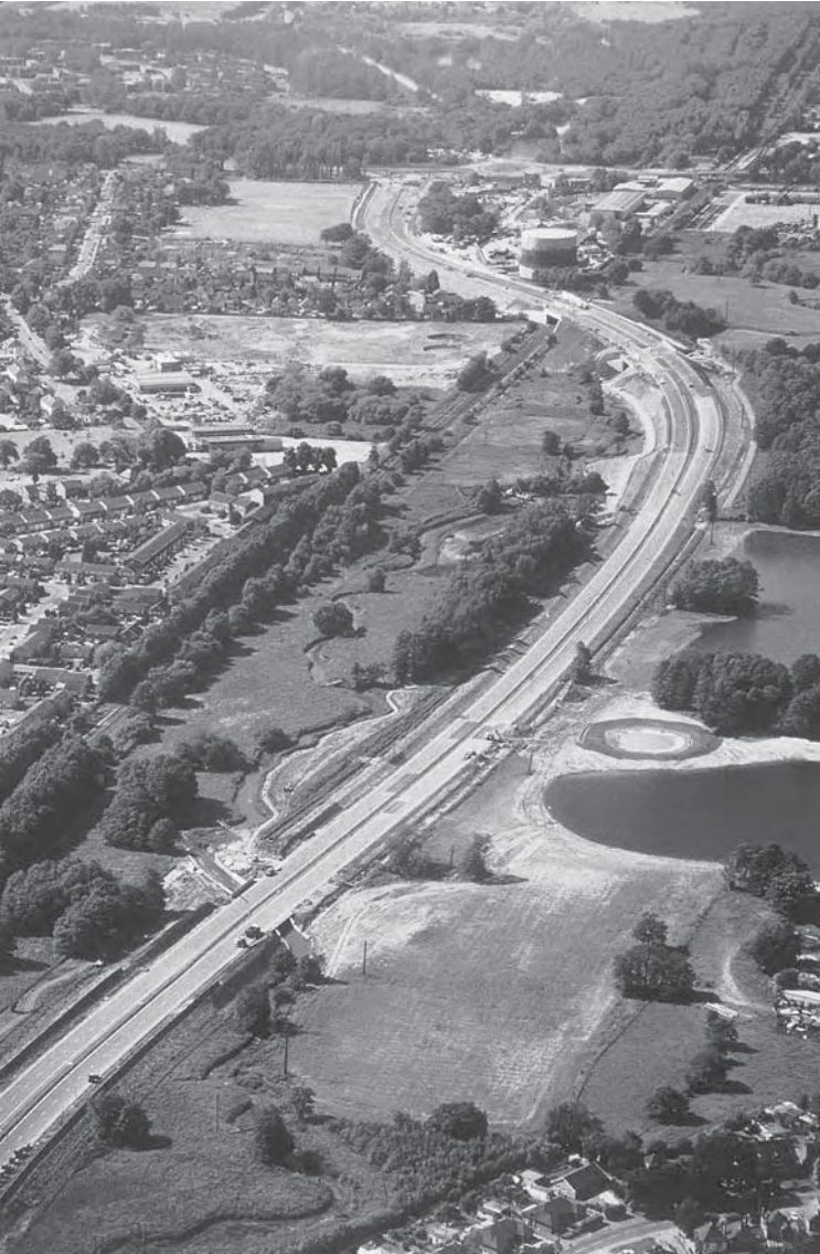
Figure 12.2 Mitigation and enhancement associated with the newly constructed Blackwater Valley Road in Surrey, completed in 1995 (photograph by A Brookes). Borrow pits used for gravel extraction (to the right of the aerial photograph) subsequently became filled with water and are important wildlife habitats and fisheries. The original river channel had been severely modified by widening, deepening and straightening over the past 100 yr or so. Whilst nearly 12 km of river channel had to be moved as a result of road construction on the floodplain, the opportunity was taken to create a more natural sinuous meandering channel on virgin floodplain, away from the road. This channel was designed to accommodate the current water and sediment discharge characteristics of the watercourse.
