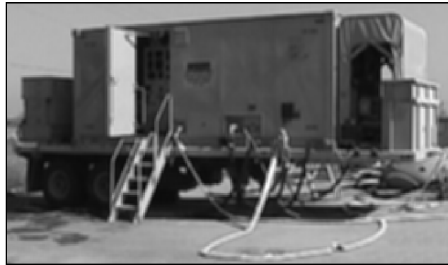
Figure 2. A trailer-mounted Reverse Osmosis Water Purification Unit (ROWPU) in operation. Source: US Army.
