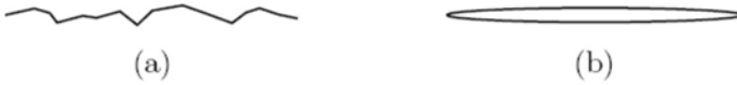
Fig. 4.4. Representation of (a) a realistic crack shape with microroughness by (b) an equivalent elliptic crack
