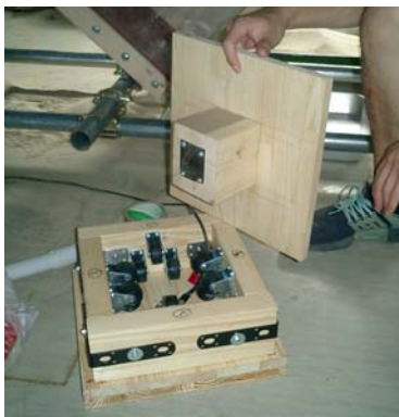
Fig. 3.5. Photo of instrument for measuring the impact force
