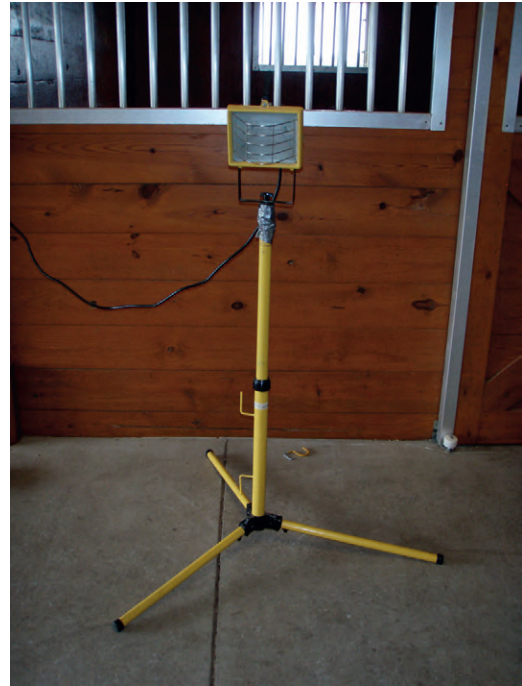
Figure 2-47. Halogen work lights can provide useful auxiliary lighting in dimly lit barns. Compact units that can be hung on a wall are readily available. A high-wattage halogen light source mounted on an adjustable tripod is ideal.
