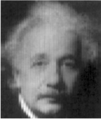
Fig. 16.1 Radiographic film irradiated with an IMRT plan, painting out a picture of Einstein with radiation
