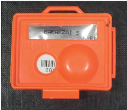
**Fig. 3.4** Radiation dosimeter
