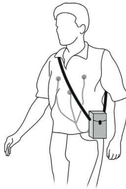
Figure 9.13 A modern electrocardiographic recorder called a Holter Monitor can record the electric field generated by the heart for 24 h or more. (Courtesy of Midmark Corporation.)
