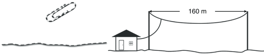
Figure 3.5 Straighten out an ordinary paperclip, and you have a 160m antenna. 160m is the wavelength (the length of one wave) corresponding to a frequency of about 2,000,000 cycles per second (abbreviated as Hz). The paperclip is seven octaves below 160m. An orchestra typically uses instruments over eight octaves.
