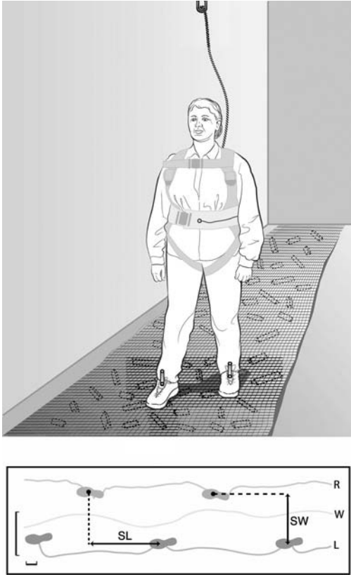
Figure 1 The irregular walkway PN patients traversed under low light conditions. Note the optoelectronic markers over the midline of the trunk and the ankles. Schematic diagram demonstrates the manner in which step width and step length were determined.
