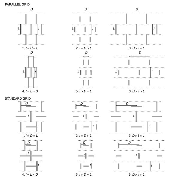
**Fig. 12.6** Manipulating trench length (L), interval (I) and distance (D) can lead to a potentially endless array of systematic trenching patterns (Source: Verhagen and Borsboom 2009)
