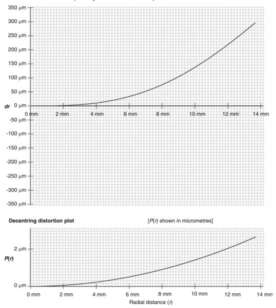
Gaussian radial distortion plot [dr shown in micrometres]
