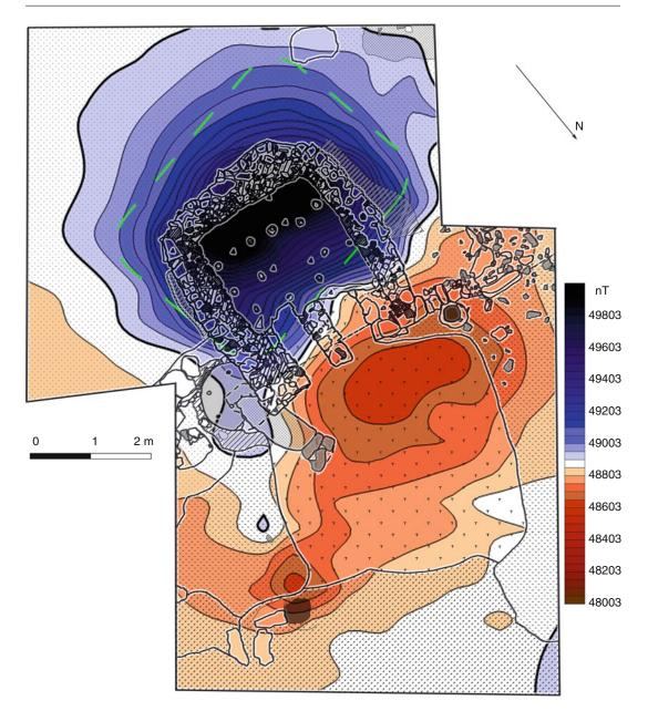
Fig. 7.10 A pottery kiln from the eighth to tenth century AD in Crimea was detected with an anomaly amplitude of more than 800 nT
