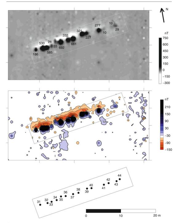
**Fig. 7.9** Blocks of slag below former iron furnaces in Denmark create a line of magnetic anomalies with highs that are usually greater than 200 nT
