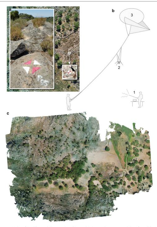
**Fig. 3.10** (a) One of the oblique aerial images taken with the Helikite platform. The insets show one of the applied ground targets and how it is rendered in the final aerial photograph (b). A schematic overview of the Helikite
