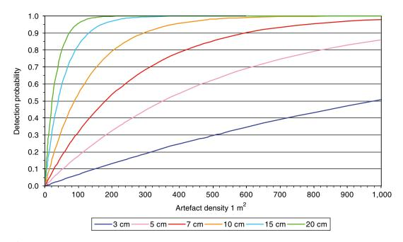
Fig. 12.10 Detection probabilities for different core diameters (Source: Tol et al. 2004, reproduced with permission)
