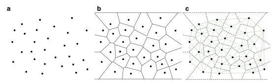
Fig. 13.9 How a TIN model is produced
