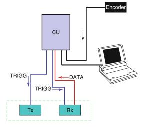
**Fig. 9.2** Basic scheme of a GPR system. *Tx* transmitter, *Rx* receiver, *CU* control unit, *TRIGG* trigger
