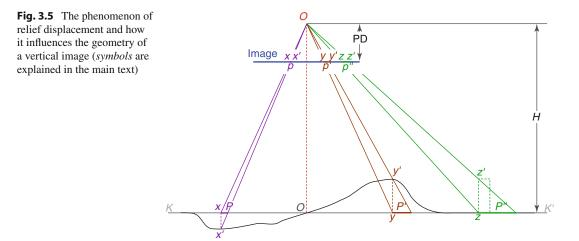
(because its projection is a perfect orthogonal projection), relief displacement is always radial from the nadir or plumb point o. This is determined by the intersection of a vertical, constructed from the optical centre O towards the ground, and the image plane; this vertical axis is equal to the optical axis of the whole system in the case of a perfect vertical photograph – such as Fig. 3.5 (Tewinkel et al. 1966).
