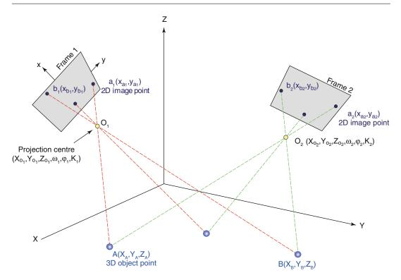
Fig. 3.2 Mapping of 3D object points onto 2D points in two aerial frame images
