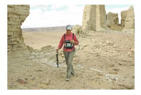
**Fig. 7.1** Doing a magnetic survey in the Fayoum Oasis with a single magnetic sensor (the *white cylinder*) that is held at a height of about 25 cm
