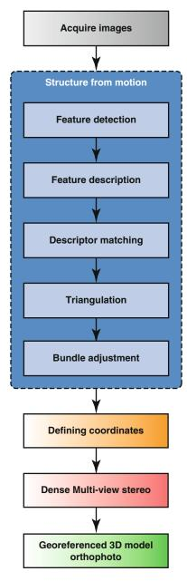
**Fig. 3.6** The individual steps of the SfM+MVS processing pipeline (terminology is explained in the text)
