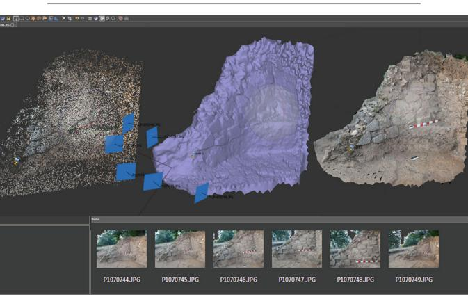
Fig. 18.2 Production of a 3D reconstruction with Agisoft
