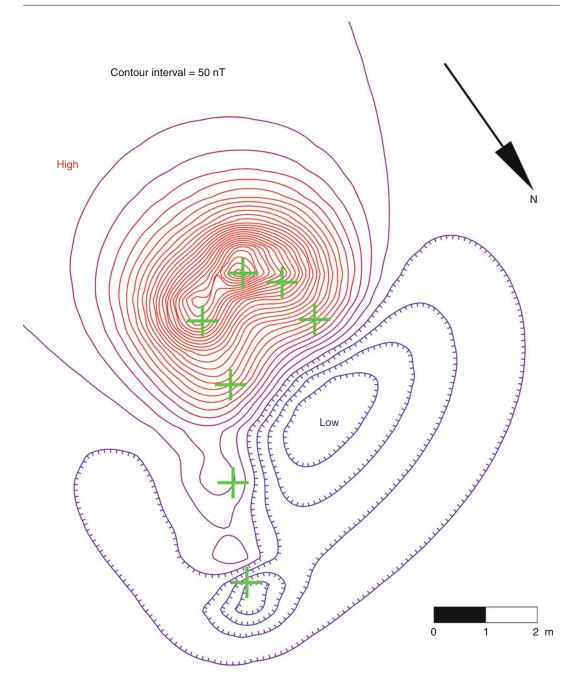
**Fig. 7.14** The calculated magnetic field of a modeling program approximates the measurements that were made on the underground kiln in Fig. 7.10
