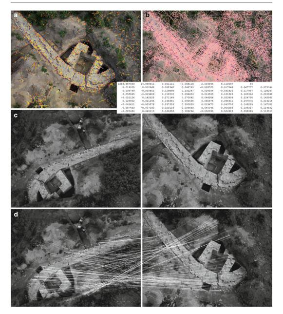
**Fig. 3.7** (a) SURF IPs computed from an airborne image using ImageJ SURF (Labun 2009). The 1,852 IPs are accompanied by their orientation vectors whose lengths indicate the strength of the computed IPs. (b) The 1,852 SURF IPs with their descriptor windows. The inset shows the vector describing one of these IPs. Computations were
