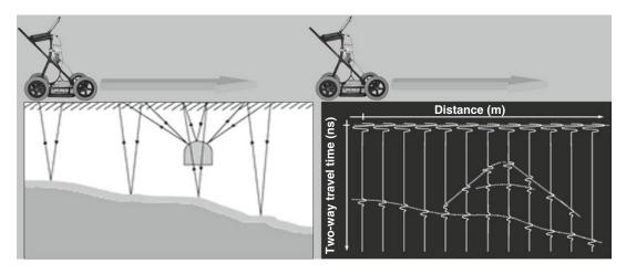
Fig. 9.1 The GPR cart is moved along a certain distance in order to equidistantly acquire reflected energy traces
