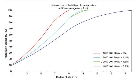
**Fig. 12.9** The effect of manipulating trench spacing and trench length on intersection probability for parallel grids while maintaining the same area coverage (Source: Verhagen and Borsboom 2009)
