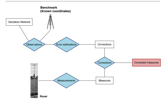
Fig. 13.4 A schematic workflow of RTK survey with a GNSS
