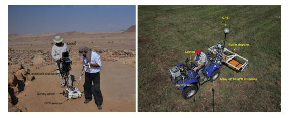
Fig. 9.3 Left single-antenna configuration for small areas. Right multi-antenna array system for large areas
