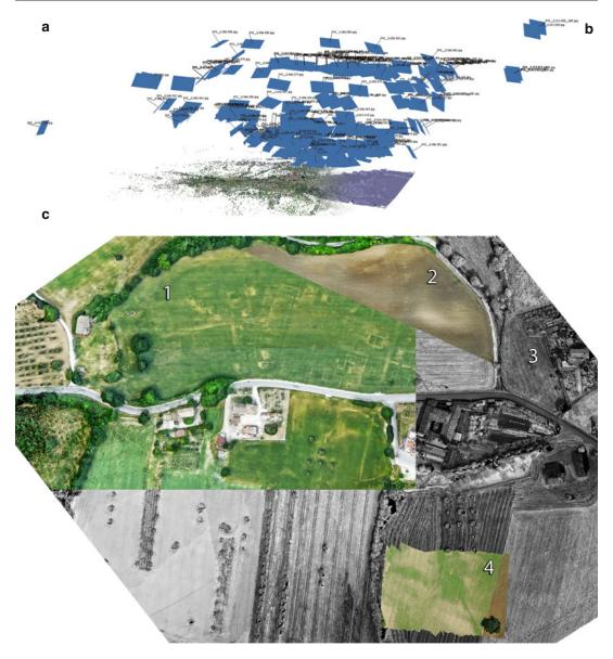
**Fig. 3.8** (a) The relative position of all 203 camera stations. (b) The extracted DSM of *Trea*. (c) The integration of several orthophotos, showing crop marks (*I*) and soil
