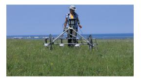
**Fig. 7.12** Four magnetic sensors (the *white cylinders*) on a cart allow an exploration of a band that is 2 m wide
