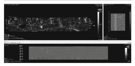
**Fig. 9.9** Interactive view of depth slice at 0.996 m depth (*top left*), perpendicular section (*top right*) and longitudinal section (*bottom*). The area is approximately 1 ha and was collected in 2 h at  $6 \text{ cm} \times 12 \text{ cm}$  resolution
