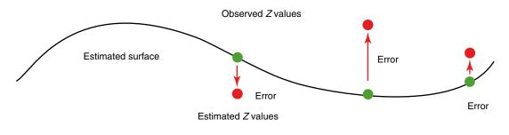
Root Mean Square Error (RMSE): Resumes the difference (error) between Observed (measured) and estimated (interpolated) *Z* values
