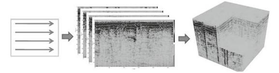
**Fig. 9.5** From *left* to *right*: Grid plot of data collection shows four parallel profiles. The raw data acquired are four B-scans. During post-processing the B-scans can be compiled into a 3D volume (or C-scan)
