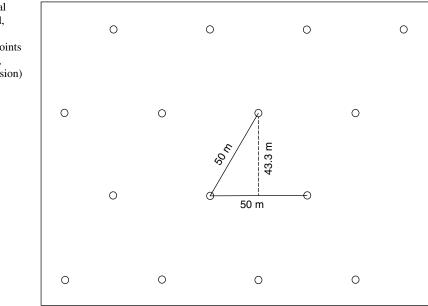
**Fig. 12.4** An equilateral triangular sampling grid, with distances of 50 m between the sampling points (Source: Tol et al. 2004, reproduced with permission)
