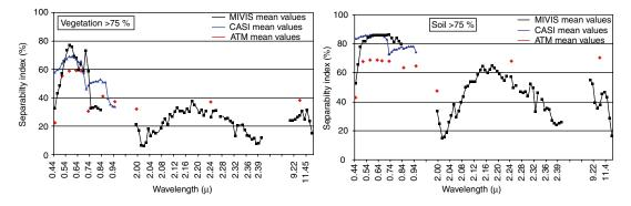
**Fig. 5.10** The mean values of SI for each ATM, CASI and MIVIS band (represented with the wavelength in microns) of all the test sites showing more than 75 % of (**a**) green crop and (**b**) bare soil end-members (Pascucci et al. 2010)
