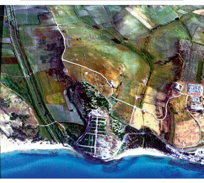
**Fig. 5.6** An example of a merged image, the combination of MIVIS image in RGB (*red* represents channel 13, *green* represents channel 7 and *blue* represents channel 1)
