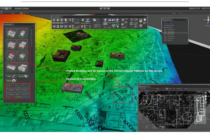
Fig. 18.3 Real-time construction editor with the library of modularised building blocks
