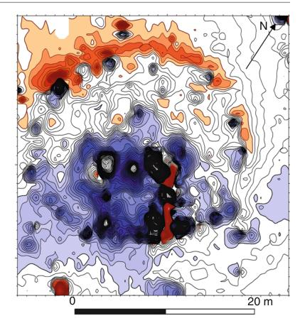
**Fig. 7.4** Granite boulders within a megalithic grave in Denmark create magnetic anomalies of 50–200 nT
