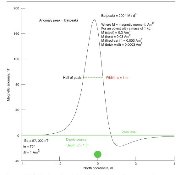
Fig. 7.13 The half-width rule approximates the depths of objects and estimates of mass are also possible
