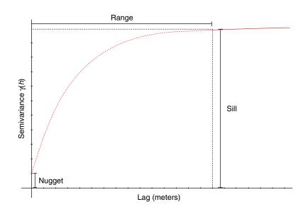
**Fig. 13.8** Representation of a theoretical variogram
