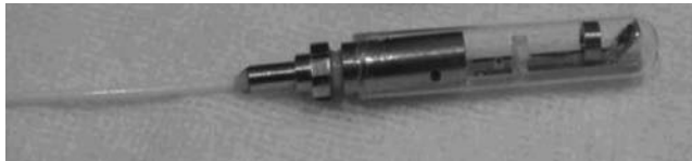
FIGURE 18.21 Endoscope probe assembled in a 5 mm glass tube.
