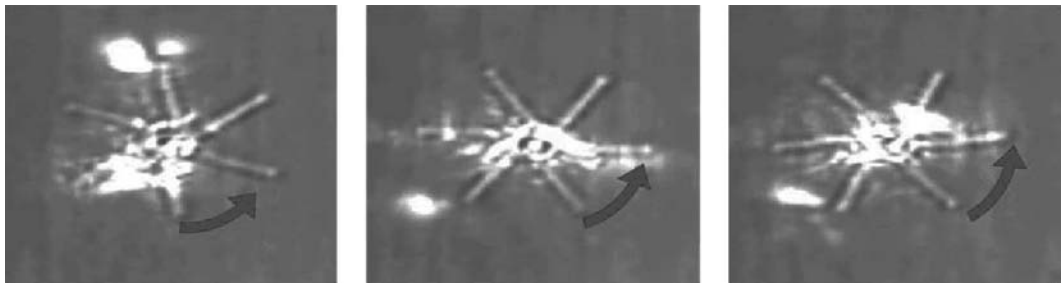
FIGURE 10.26 Sequential optical images of a rotating microrotor of type E at 2 s intervals. (Copyright (2011) The Japan Society of Applied Physics.)
