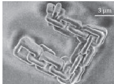
FIGURE 16.2 Three-dimensional microstructure fabricated using two-photon absorption. (Reprinted with permission from Sun, H.B. and Kawata, S., J. Lightwave Technol. , 21, 624–633. Copyright 2003, IEEE.)
