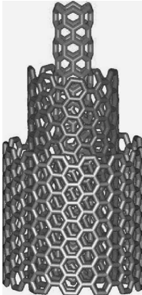
FIGURE 1.11 Structure of a multi-walled carbon nanotube (MWCNT) made up of three cylindrical shells. These types of MWCNT can have diameters up to 100 nm. (Balasubramanian, K. and Burghard, M.: Chemically functionalized carbon nanotubes. Small . 2005. 1(2). 180–192. Copyright Wiley-VCH Verlag GmbH & Co. KGaA. Reprinted with permission.)
