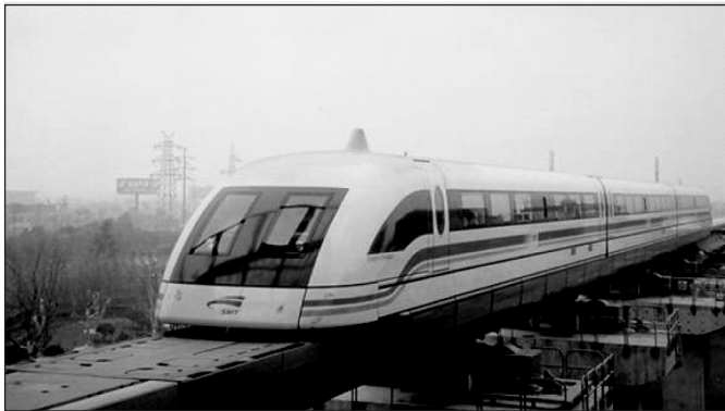
FIGURE 8 The Shanghai maglev train, Transrapid, in operation (430 km/h speed).
