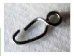
Figure 13.34 Separating spring.
