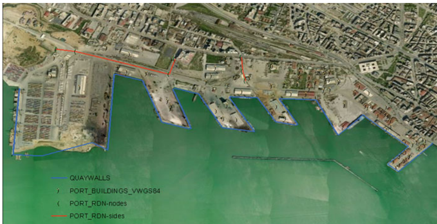
Fig. 12.7 Internal road network of Thessaloniki’s port
