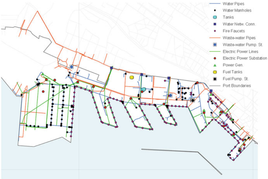
Fig. 12.5 Water supply, waste-water, fire-fighting, electric power and fuel supply systems of Thessaloniki's port
