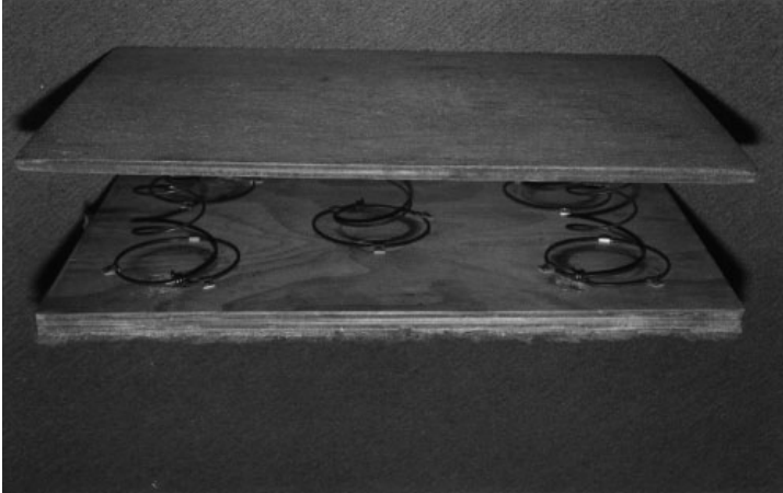
Figure A4.4: Balance board with upholstery springs
