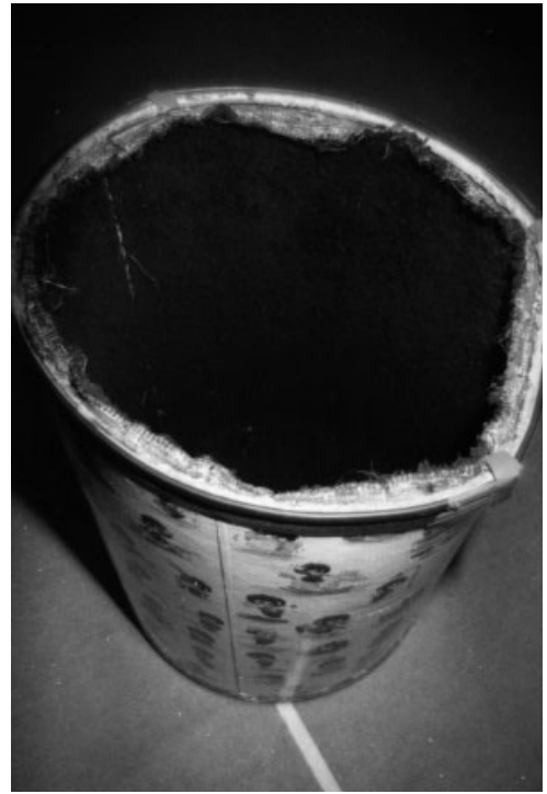
Figure A4.7: Barrel, showing the inside lined with carpet
