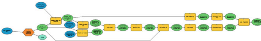
Fig. 7 Screenshot of an ESRI ArcMap model that begins with point data of fortress occupations, iterates a rasterized viewshed for each one, converts the positive values into polygon vectors, and re-attaches data such as architecture type, dates of occupation, and affiliation for each viewshed
