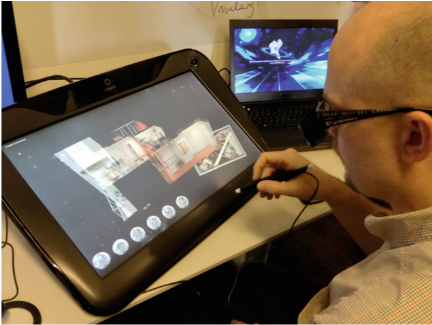
Fig. 7 Holographic virtual reality collaborative platform managed by a 3D stylus. Here the users can explore the potential of proprioception (a sense of how our bodies are positioned) and eye-tracking in the virtual exploration of archaeological artifacts
