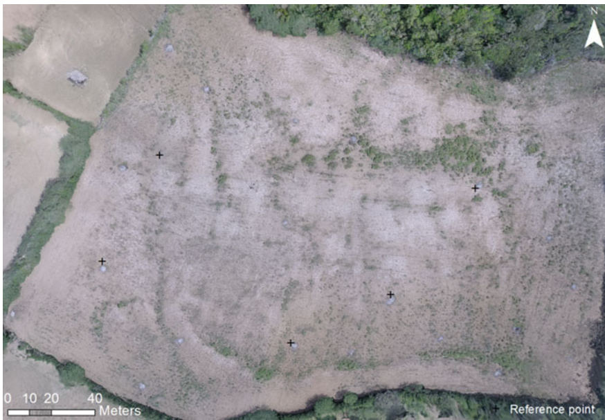
Fig. 8 Orthophoto of El Manantial using 240 images and ground control points
