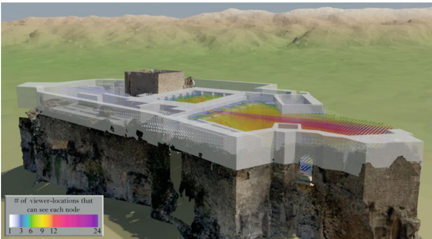
Fig. 14 A rendering of the Montesa modeling project. The colored voxels represent the number of times a hypothetical viewer walking from the gate (lower right) through the cloister (center) could see each unit of space. The experiment allows the viewer to look in all directions every two feet along their path
