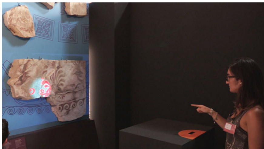
Fig. 12 The magic flashlight , presented in the Keys2Rome exhibition. The user moves his finger upon the Leap Sensor, this movement is tracked in order to project the original colour on the archaeological fragment. INRIA, French National Institute for Computer Science and Applied Mathematics, 2014
