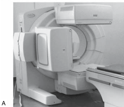
Figure 10.1. A: A three-head gamma camera-based positron emission tomography (GCPET) system (Philips Irix 3000). The three heads can be placed at different gantry angles with respect to each other and can be used for both routine SPECT as well as for coincidence imaging. B: A schematic representation of the coincidence circuit used in a GCPET system. For a coincidence event to be detected, the two photons must be detected within the 15-ns timing window and should lie within the specified energy range.
