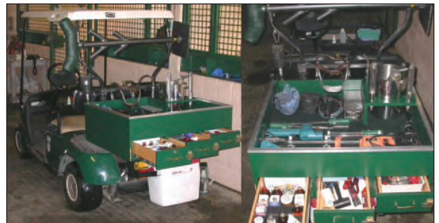
Figure 15.4. An electric golf cart converted to a mobile equine dental station (TA Banner, DVM, Gaines)
