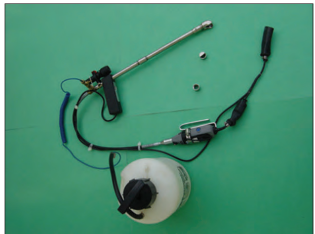
Figure 15.37. Variable-speed flexible-shaft tooth grinder with long shaft and compact, guarded head. This unit has a built-in water irrigation unit and light (Jupiter Vete
