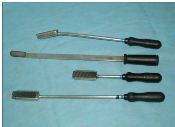
Figure 15.29. Four basic floats used to perform routine dental prophylaxis. From top to bottom: (1) round medium-length shaft, 20° downward-angled, box head float with rubber handle, (2) flat long-shaft, 10° upward-angled, bonded head float with neoprene handle, (3) round, short-shaft, straight, box head float with rubber handle, and (4) round, long-shaft, straight box
