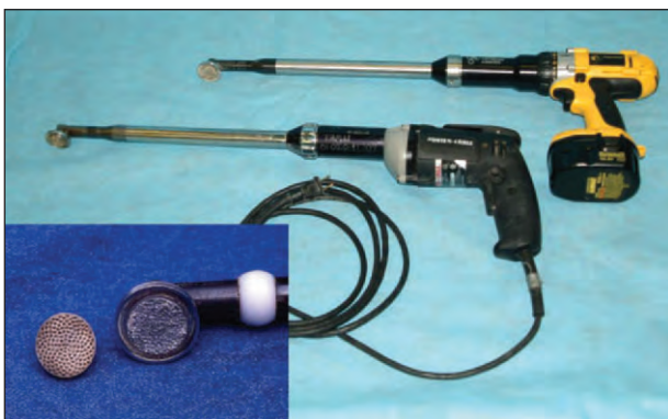
Figure 15.38. Battery and electric-powered disk burr (PowerFloat ® ). The carbide chip or diamond grit rotary disk head is guarded by a stainless steel lip (D & B Equine Enterprises, Inc., Calgary, Alberta, Canada).
