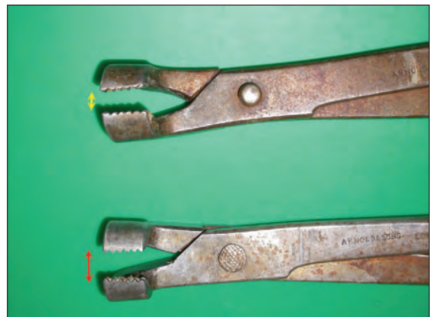
Figure 18.21. Different jaw widths are necessary to enable a good contact with both mandibular and ma
