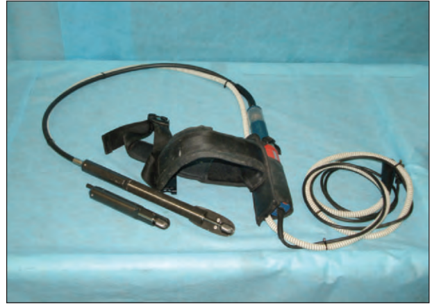
Figure 15.36. Rotary dental grinder constructed from a Suhmer motor with clutch, a variety of guards, vacuum system to remove dental dust and various style heads and burrs (Carbide Products Co., Torrance, CA, USA).
