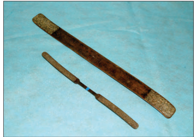
Figure 15.32. A steel S-shaped double end file and large carbide grit table float.
