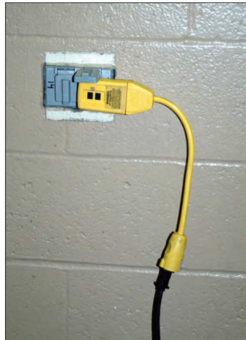
Figure 15.39. An extension cord with a ground fault circuit interrupter (GFI) incorporated in the plug. A GFI should be used whenever electric tools are used for dentistry to prevent the possibility of electric shock.
