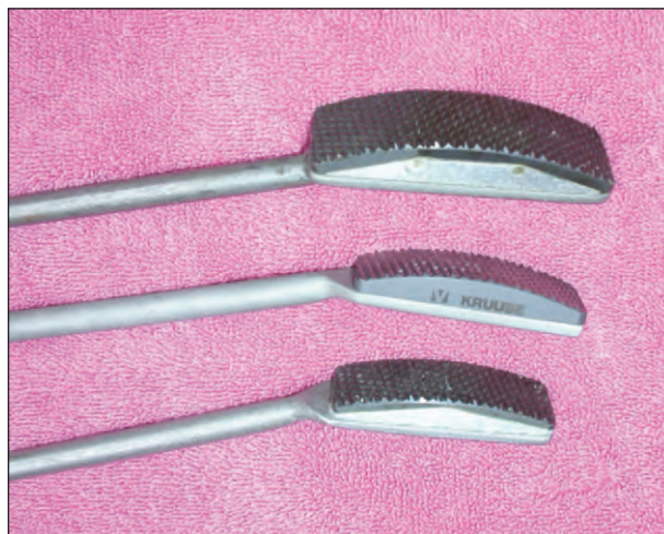
Figure 15.28. An innovation in solid tungsten carbide float head and blade design. These convex blades are very useful in reducing dental overgrowths (Kruuse Worldwide, Marslev, Denmark).
