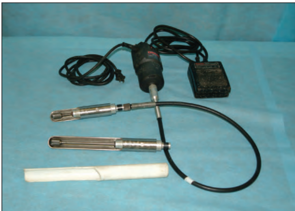
Figure 15.35. A flex-shaft with variable-speed foot pedal, Dremel ® motor tool modified to perform dental corrective procedures. The white PVC pipe guard is homemade. The stainless steel guard and extended shaft burrs have been designed for corrective procedures on incisors, canines and premolars (Dremel ® , Racine, WI, USA; Harlton's Equine Dental Specialties, Columbus, OH, USA).
