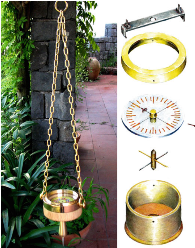
Fig. 5.5 Reconstruction of a suspended compass with chain ( right ) and image of exploded view of the compass, both by the authors
