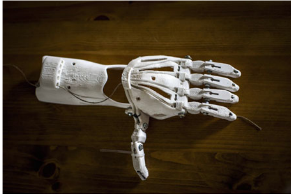
Fig. 4.13 A 3D printed hand prosthetic. Image Source http://www.pixabay.com/
