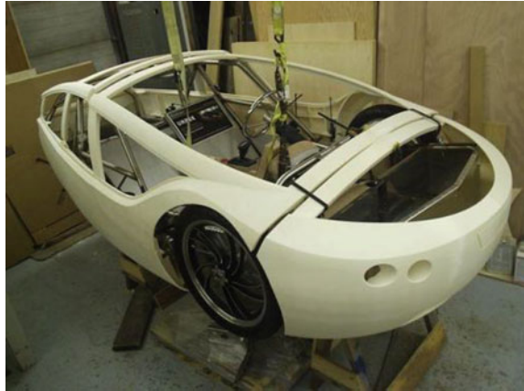
Fig. 2.13 3D printed URBEE2 car body. Image Source KOR Ecologic Inc.
