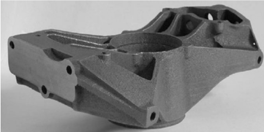
Fig. 2.11 A race car upright made by EBM. Image Source Petrovic et al. (2011)
