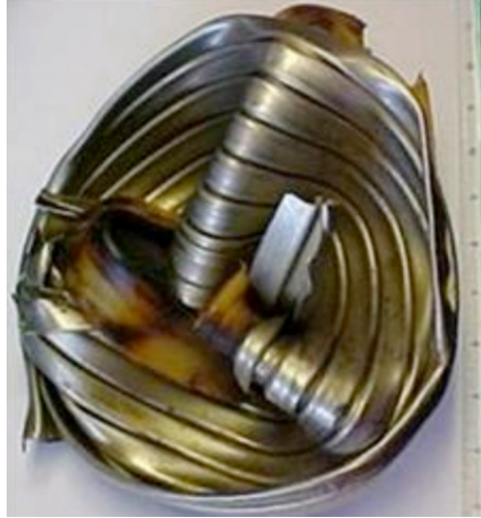
FIGURE 5.3 Collapsed Carcass due to Hydrostatic Pressure. Source: Out [6]. (For color version of this figure, the reader is referred to the online version of this book.)
