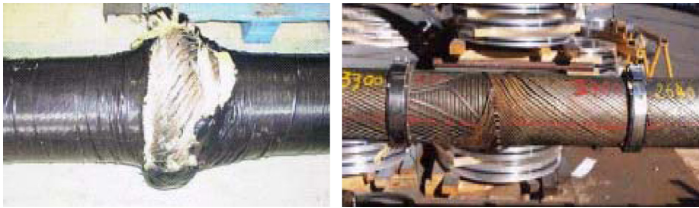
FIGURE 5.5 Tensile Armor Layers' Failure Modes , Source: O'Brien [7]. (For color version of this figure, the reader is referred to the online version of this book.)
