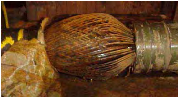
FIGURE 5.6 Birdcaging . Source: Clevelario [8]. (For color version of this figure, the reader is referred to the online version of this book.)
