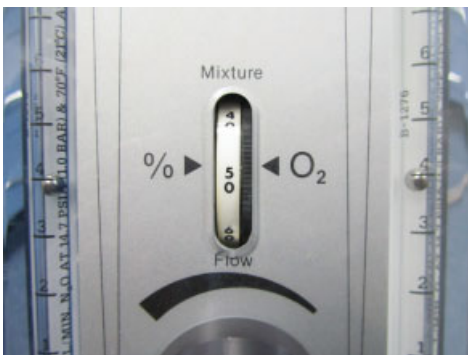
Figure 5.16 Dial at 50% oxygen and nitrous oxide (centre) and calibrated balls at 4L/min for both gases (left and right).
