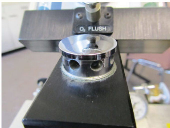
Figure 5.23 Air entrainment valve.
