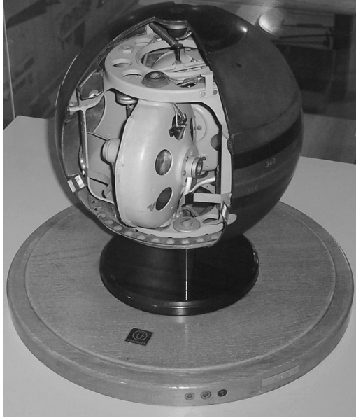
Figure 21.2 Cutaway of Anschütz gyrocompass.
