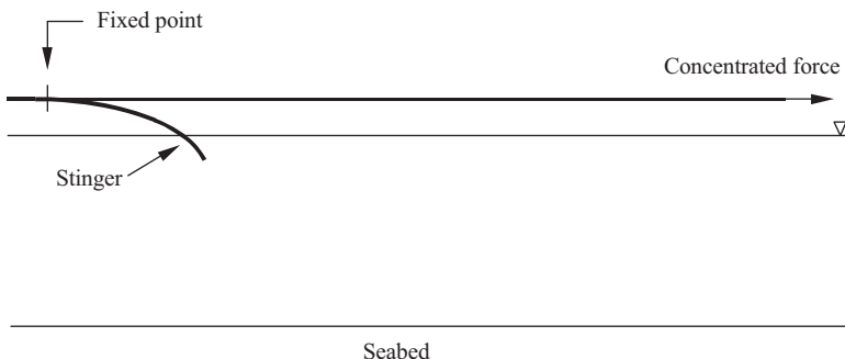
Figure 33.30 Pipeline initial configuration and load step 1.
