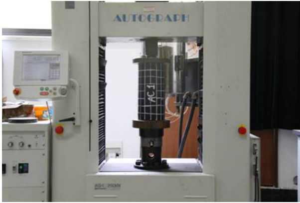
Figure 26.7 Axial compressive test arrangement. (For color version of this figure, the reader is referred to the online version of this book.)
