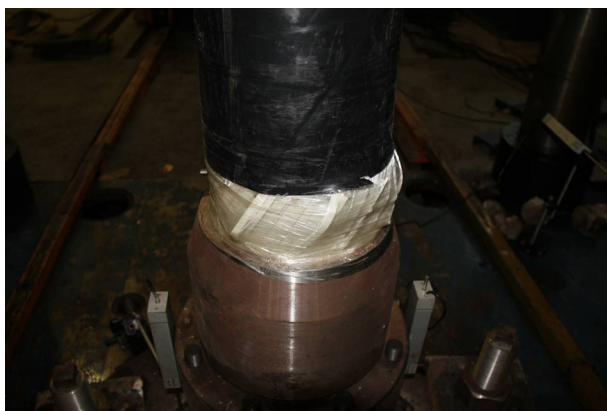
Figure 26.3 Rupture of the glass-fibers in Mode 1. (For color version of this figure, the reader is referred to the online version of this book.)
