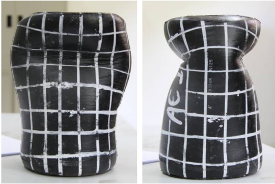
b) Failure mode shape of AC 1
