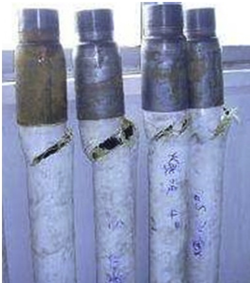
Figure 27.2 Burst samples after testing. (For color version of this figure, the reader is referred to the online version of this book.)
