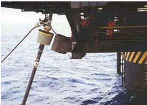
Figure 26-9 Riser Hang-Off Location
