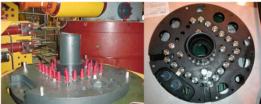
Figure 7-12 Typical SCMMB (Courtesy of FMC)
