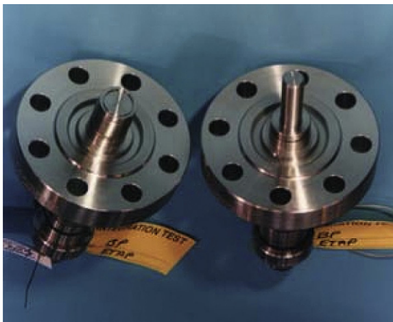
Figure 7-21 Temperature Transducers (TT)
