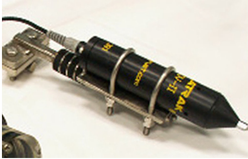
Figure 23-2 Polatrak ROVII Tip-Contact CP Probe (Courtesy of Deepwater Corrosion Services, Inc. [6])
