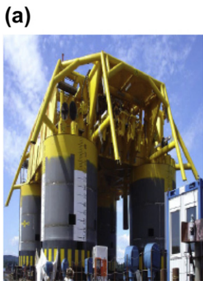
Wellhead Protection Frame
