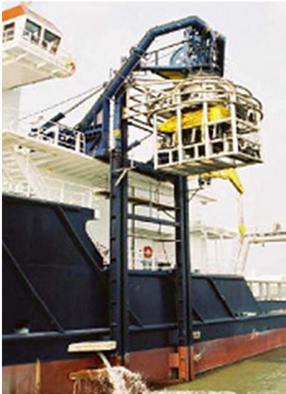
Figure 23-7 Guide Rail System [10]
