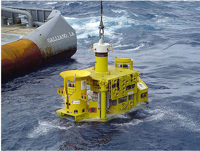
Figure 6-12 A Subsea Tree Being Deployed [5]
