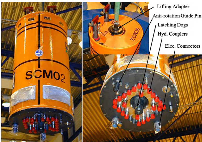
Figure 7-13 Typical SCM (Courtesy of FMC)
