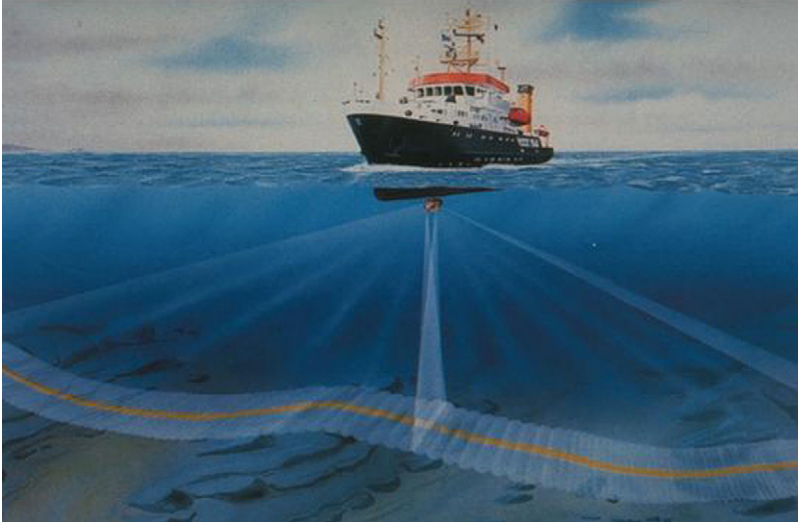
Figure 4-3 MBES Working Model [5]
