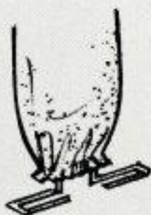
An alternate method of bending coat hanger wire and nailing the ends to a base.
