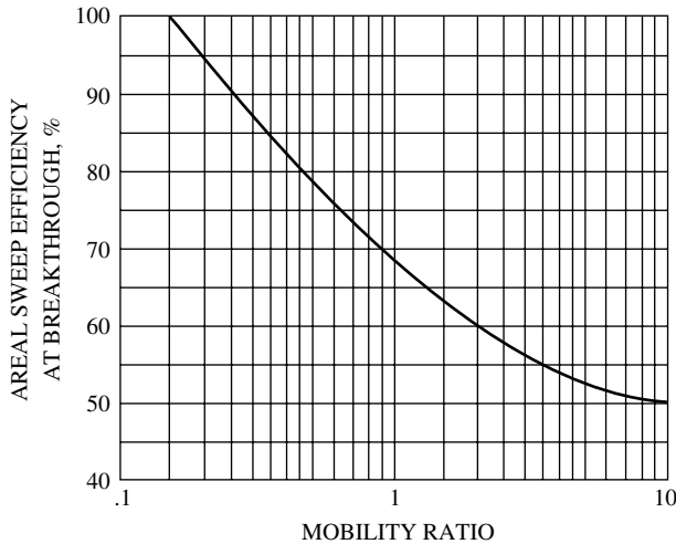
Figure 14-35. Areal sweep efficiency at breakthrough. (Permission to publish by the Society of Petroleum Engineers.)
